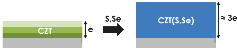
Figure II.9: Schematic illustration (cross-section) of volume expansion.
