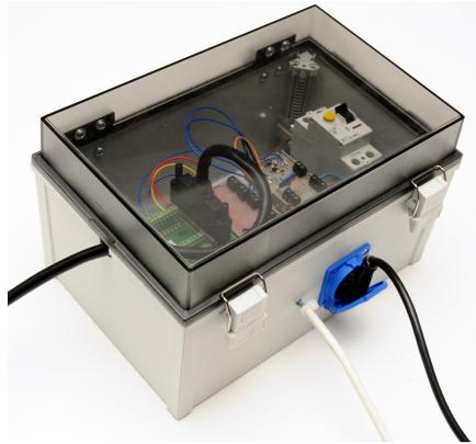
Figure 4.14 – One Phase measurement box. The box can be plugged directly between the appliance and the power outlet.
