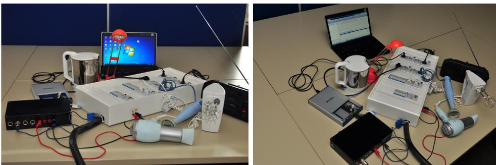
(a) The whole system with different appliances. (b) Pc, ADC, measurement box 1 and switching detection box.
