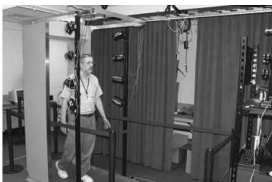
Figure 3-11: An illustration of the concept of IOM system [25]. The camera is visible at the far right of the figure.
