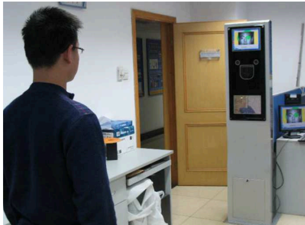
Figure 3-13: Iris acquisition at a stand-off distance of 3 meters [28].
