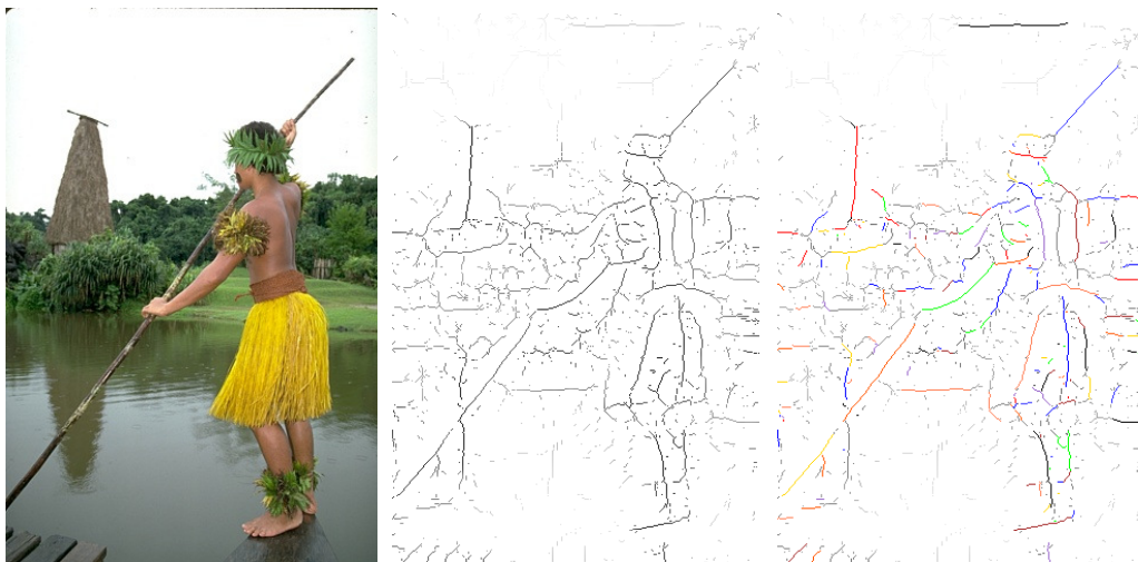
FIGURE 2.29 – From left to right : Original image, symmetry response without grouping, grouping 200 most salient contours (better viewed magnified and in color).
