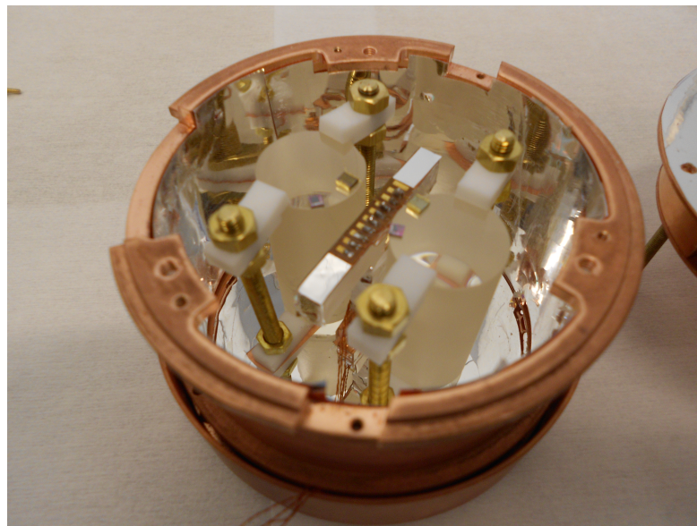
FIGURE 6.22: Picture of the detector. The two crystals are placed symmetrically with respect the holder structure in order to avoid systematics in the light collection. One ZnMoO 4 crystal is doped with W, the other is not.
