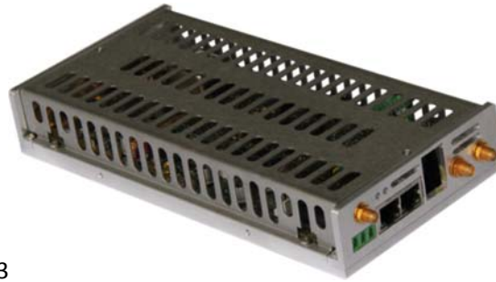
Figure 4.10 – Module integrating the Signal Generator and the pre-distorter.
