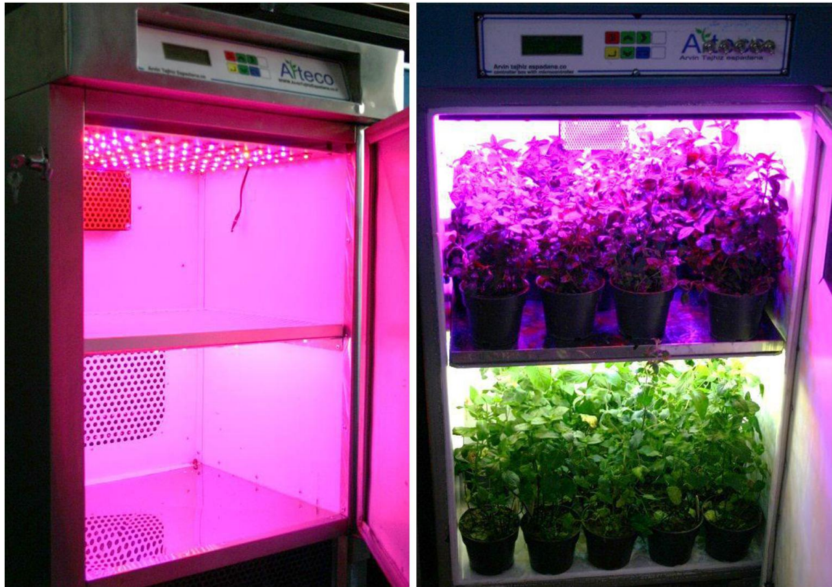
Figure 7.1. Constructed light emitting diode (LED) incubator with mint plants grown under irradiation platform. This growth chamber is in size of 1.0 width×0.6 depth×1.5 m height, equipped with microcontroller for setting the plant growth parameters of light, temperature and humidity to support plant superior growth.
