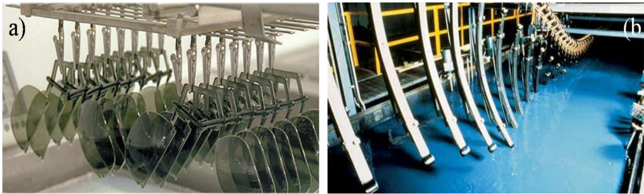
Figure. II-2 (a) Parallel dip-coating of several lenses with an antireflective-antifogging coating (image from North American Coating Laboratories® website) . (b) Conveyor-dip-coating system for continuous coating of leaf springs (image from Product Finishing website®)
