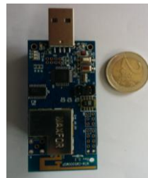
Figure. 4.2.1. Example of a resource constrained node used in smart spaces
