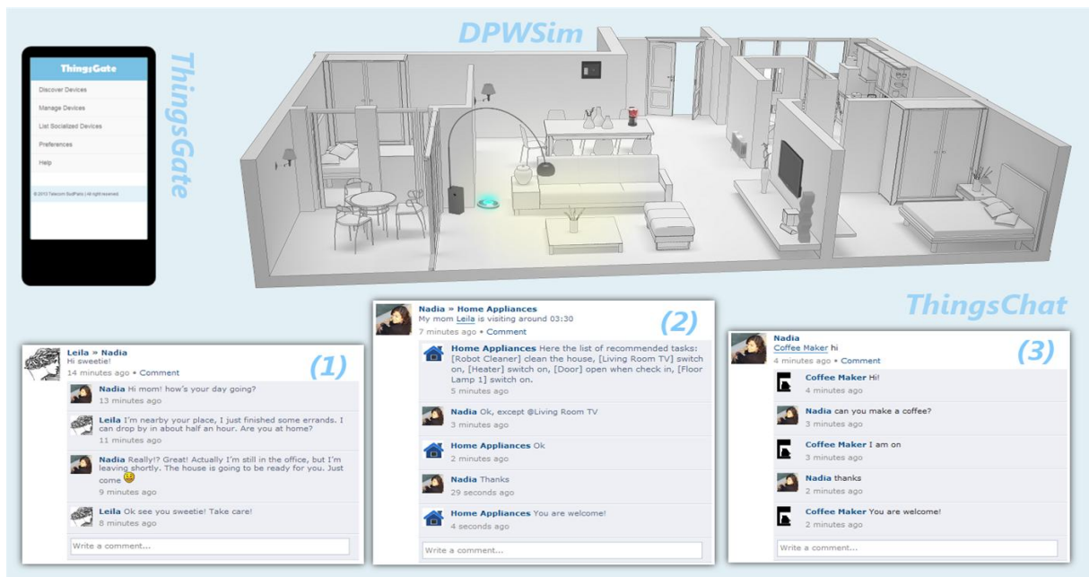
Figure 4.1.7. ThingsChat. ThingsGate is accessed by using smartphone via the mobile Web interface to discover and manage devices at virtual home of DPWS devices created in DPWSim. Below are different ways for the communication between people and devices. (i) There is a user Nadia sending Home Appliances group on ThingsChat to ask for receiving her mother Leila who is coming home while Nadia is still at the office. (ii) InRe accesses Nadia and Leila profile to recommend a list of services to be done at home, i.e., cleaning, opening the external gate, etc. (iii) Nadia accepts then most of the recommended tasks except the TV to be switched on. She also can directly chat with the coffee maker to prepare a coffee when her mother arrives.
