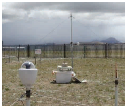
Figure 4.1: Instrument set up to record the hemispherical images (front) and net radiation instrument to record the radiative fluxes (back) at the NamCo station
