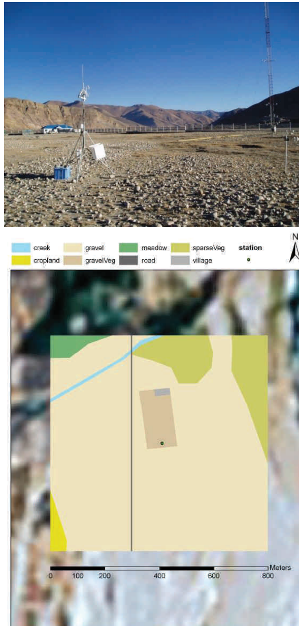
Figure 2.11: Picture of the Qomolangma site (top) and land cover map of the surroundings (bottom) from Babel et al. (2011)
