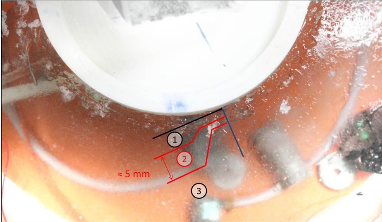
Figure 3.11: Photography of the ice layer during one realization of the laboratory Couette flow experiment showing the main fault (2) of mean width  $\approx 5$  mm, between a thin region of "fast" ice (1) along the inner rotating disk and a large motionless region (3). *Credit: V. Pellisier.*
