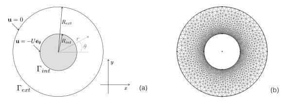
Figure 3.7: (a) Domain and boundary conditions for the annular Couette flow problem, in both the no-damage (section 3.3) and full Maxwell-EB (section 3.4) simulations. (b) Finite element mesh used in the full Maxwell-EB Couette flow simulations (section 3.4). The element size is a function of the radius r and is set as  $\Delta x(r) = \frac{R_{ext}}{N}(r)^2$ , with N = 10.
