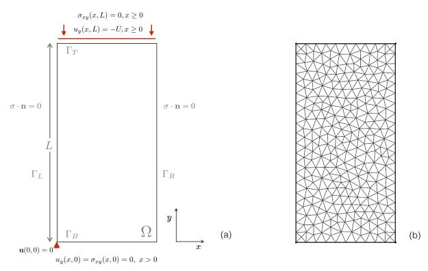
Figure 2.7: (a) Domain and boundary conditions for the uniaxial compression experiment. (b) Example of finite element mesh with N = 10.
