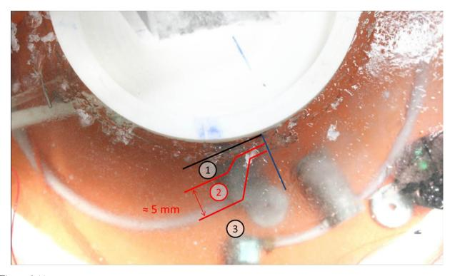
Figure 3.11: Photography of the ice layer during one realization of the laboratory Couette flow experiment showing the main fault (2) of mean width  $\approx 5$  mm, between a thin region of "fast" ice (1) along the inner rotating disk and a large motionless region (3). Credit: V. Pellisier.
