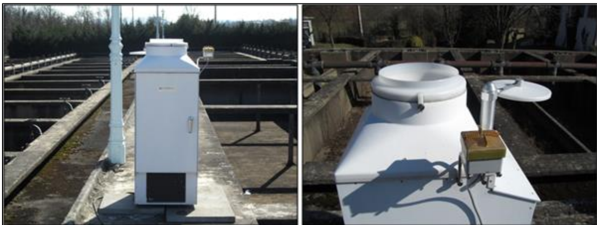
Fig.I-24: Eigenbrodt Automatic Precipitation Sampler NSA 181 with an aperture of 614cm 2 , which opens/closes automatically during and after any rainfall events
