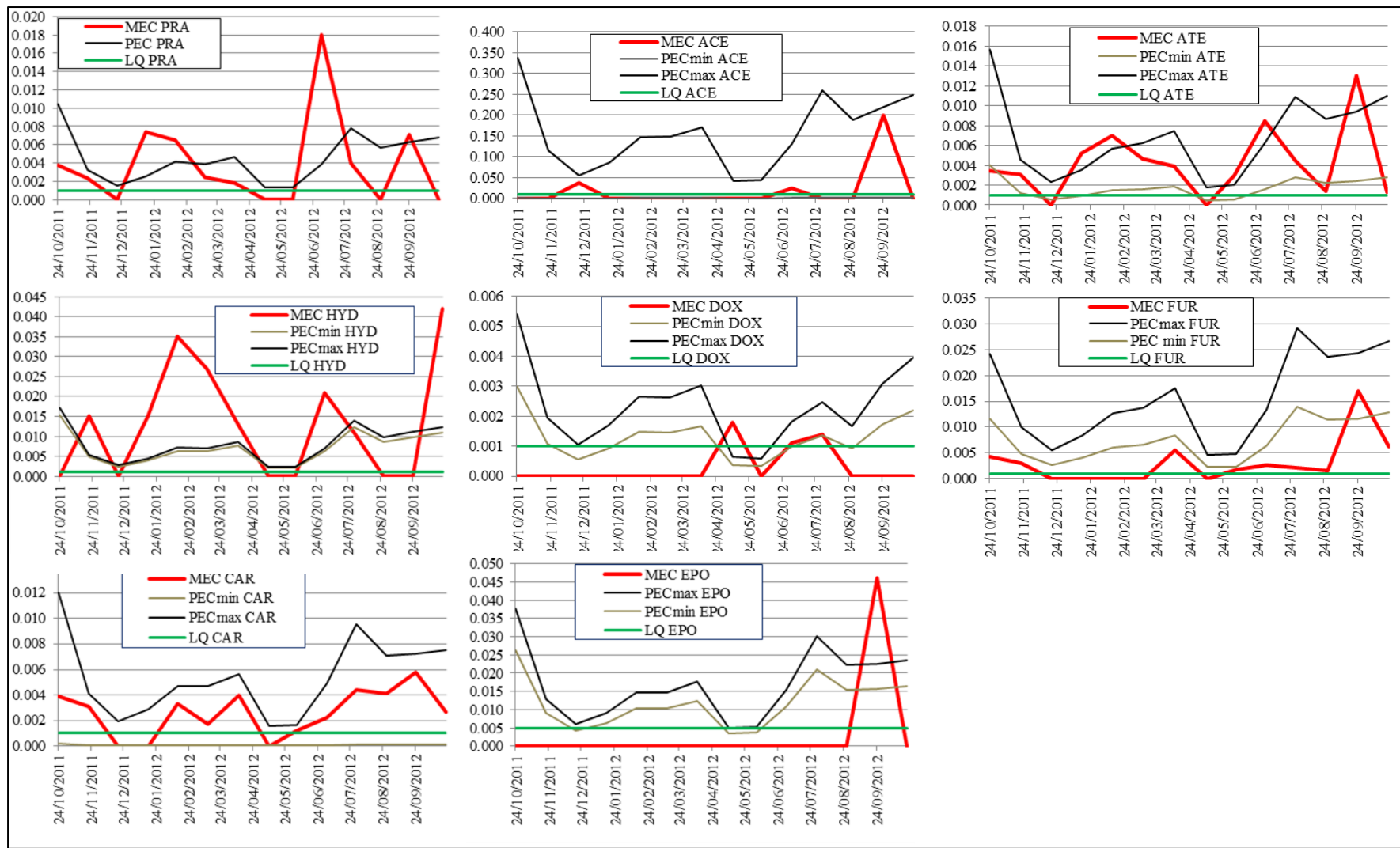
Fig.III-14: Temporal evolution of MECs (Measured Environmental Concentrations) and PECs (Predicted Environmental Concentrations). PECmax and PECmin are the maximum and minimum 3 value of PECs when data and pharmacokinetic parameters are available, LQ is Limit of Quantification.
