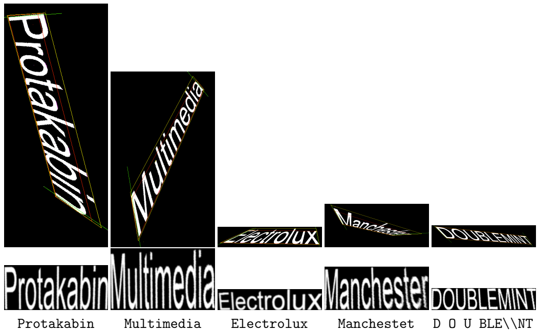
Fig. 11: Rectification results on text strings of ten characters: original image (top), text rectification result (middle) and OCR transcription using Tesseract (bottom).
