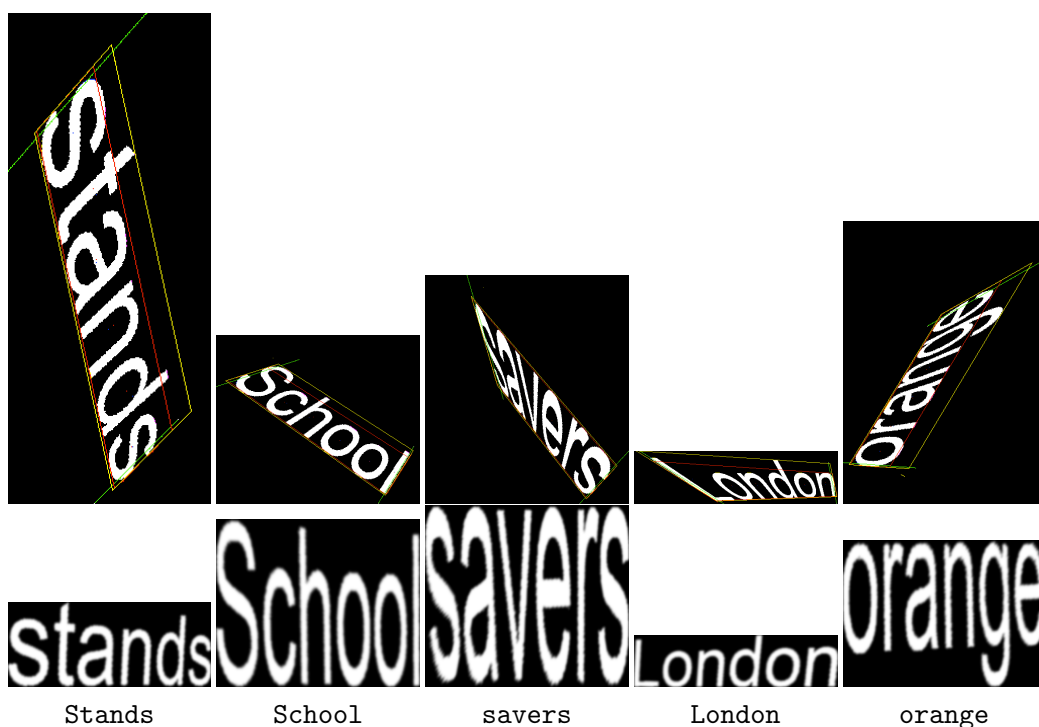
Fig. 7: Rectification results on text strings of six characters: original image (top), text rectification result (middle) and OCR transcription using Tesseract (bottom).
