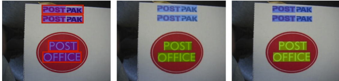
Fig. 5.5: One-to-many matching examples; left: GT (red rectangle) and the detection (solid purple rectangle); center (ICDAR 2013) and right (EvalTex): mismatched GT objects (solid red rectangles), one-to-one matched GT areas (solid green rectangles), many-to-one matched GT areas (solid yellow rectangles), one-to-many matched GT areas (solid blue rectangles).
