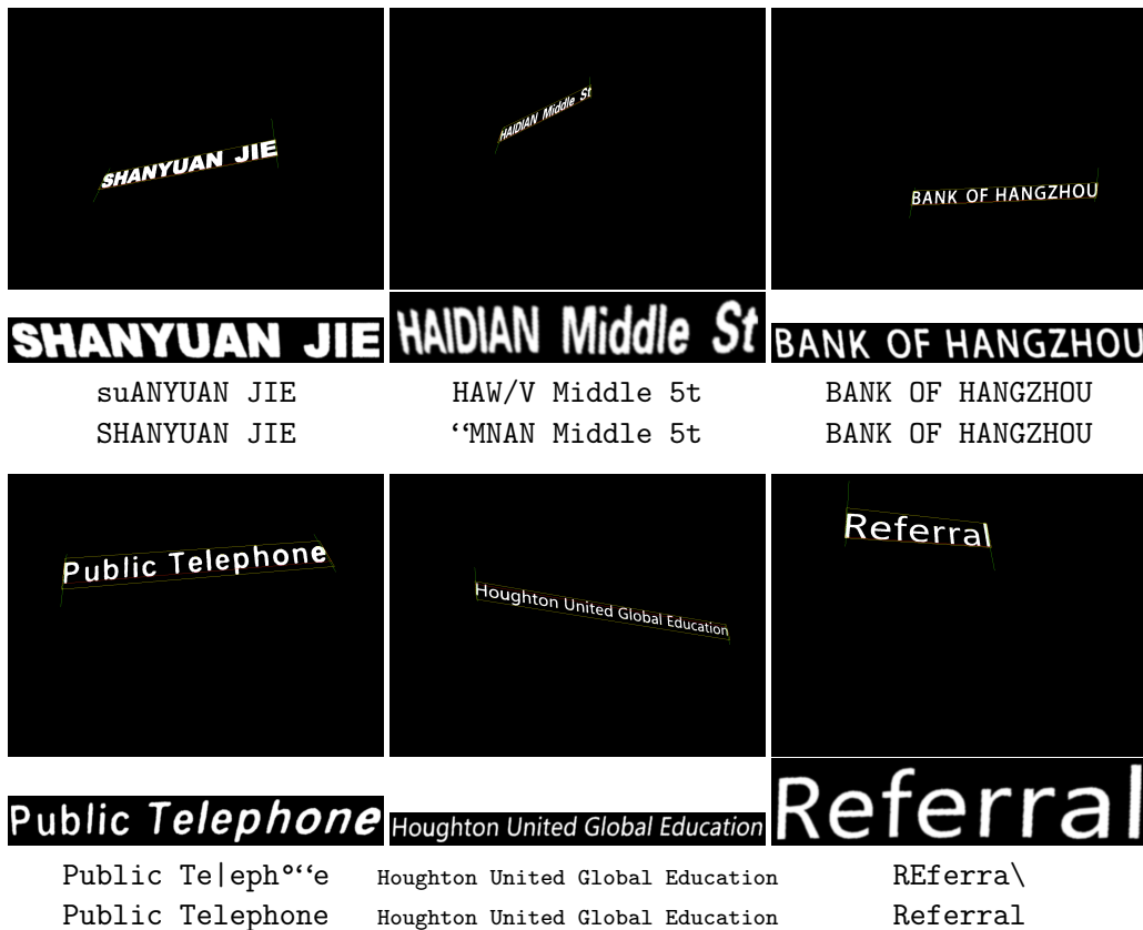
Fig. 22: Similarity of OCR recognition before and after the rectification process: original image (top), text rectification result (middle), OCR transcription before the rectification and OCR transcription after the rectification using Tesseract (bottom).
