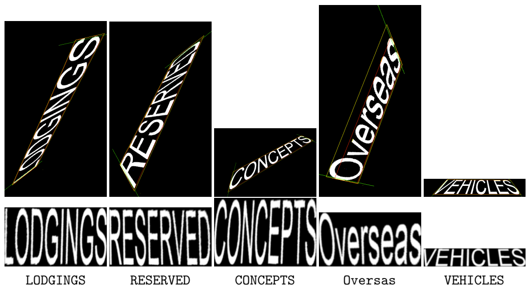
Fig. 9: Rectification results on text strings of eight characters: original image (top), text rectification result (middle) and OCR transcription using Tesseract (bottom).
