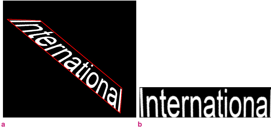
Fig. 11: Perspective distortion rectification: (a) bounding quadrangle estimation; (b) rectified text.
