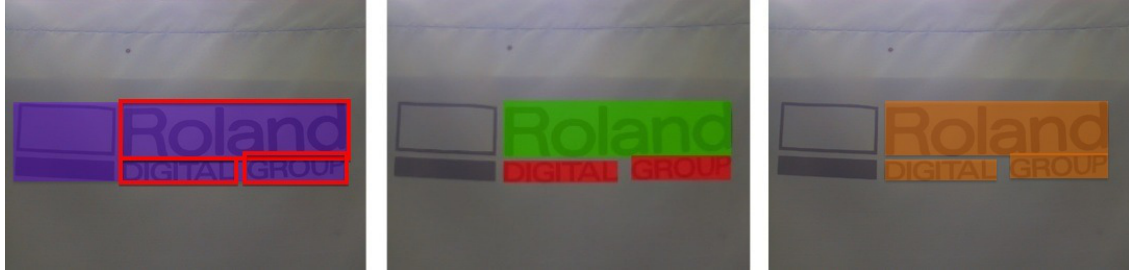
Fig. 5.6: Many-to-one matching examples; left: GT (red rectangle) and the detection (solid purple rectangle); center (ICDAR 2013) and right (EvalTex): mismatched GT objects (solid red rectangles), one-to-one matched GT areas (solid green rectangles), many-to-one matched GT areas (solid yellow rectangles), one-to-many matched GT areas (solid blue rectangles).
