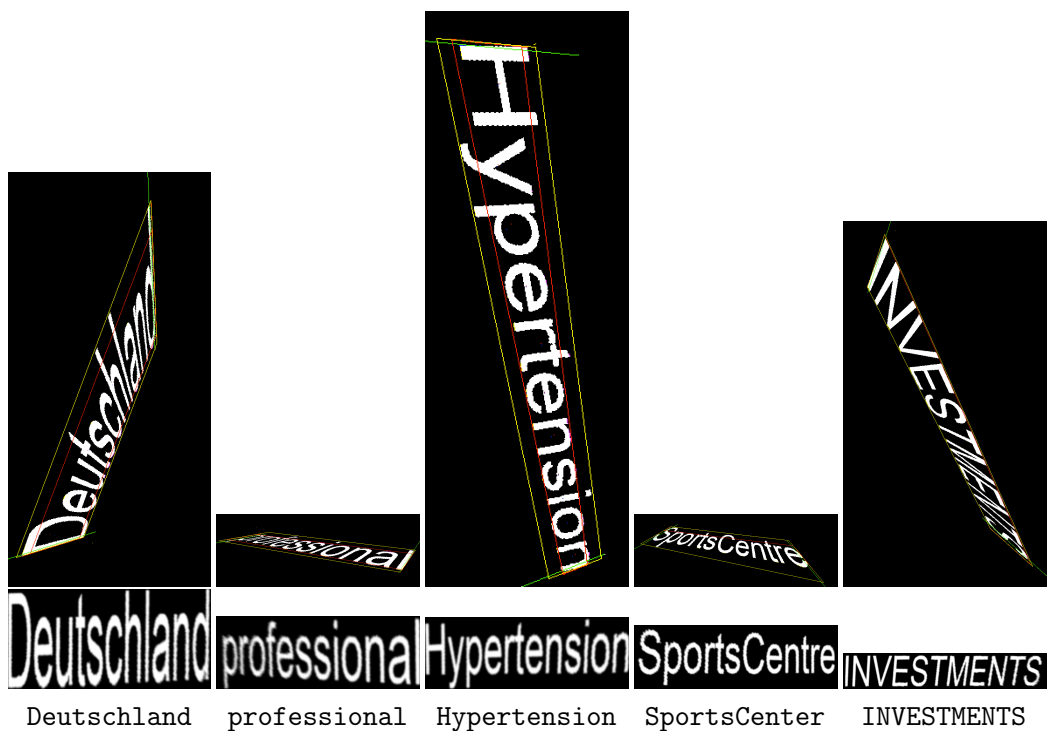
Fig. 12: Rectification results on text strings of more than ten characters: original image (top), text rectification result (middle) and OCR transcription using Tesseract (bottom).
