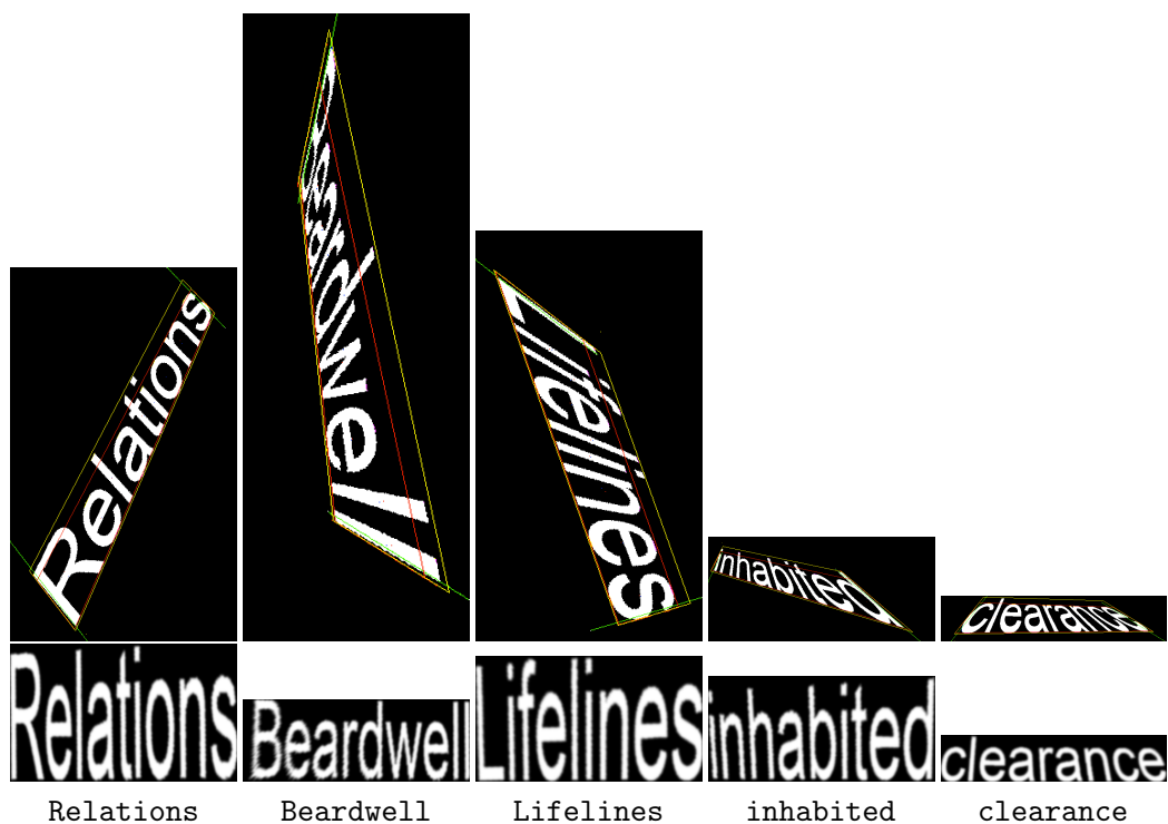
Fig. 10: Rectification results on text strings of nine characters: original image (top), text rectification result (middle) and OCR transcription using Tesseract (bottom).
