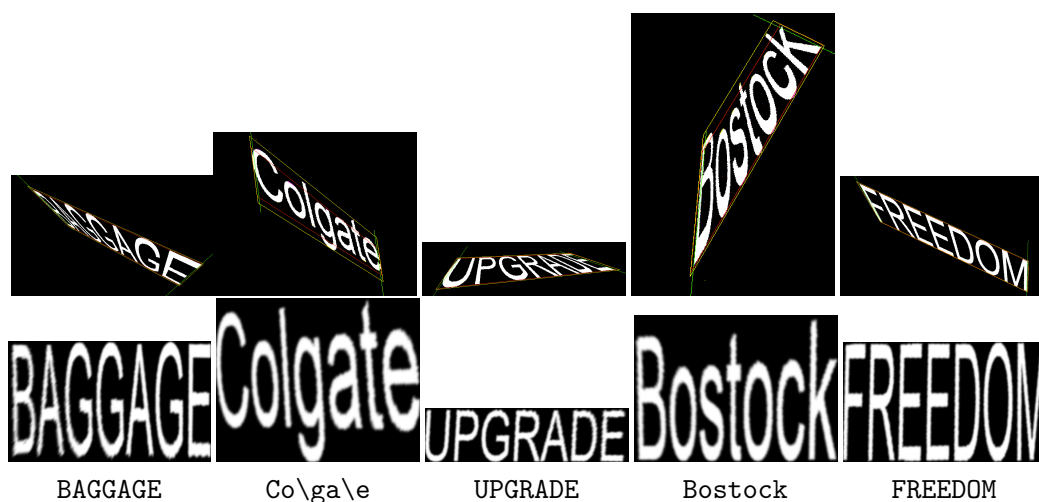
Fig. 8: Rectification results on text strings of seven characters: original image (top), text rectification result (middle) and OCR transcription using Tesseract (bottom).
