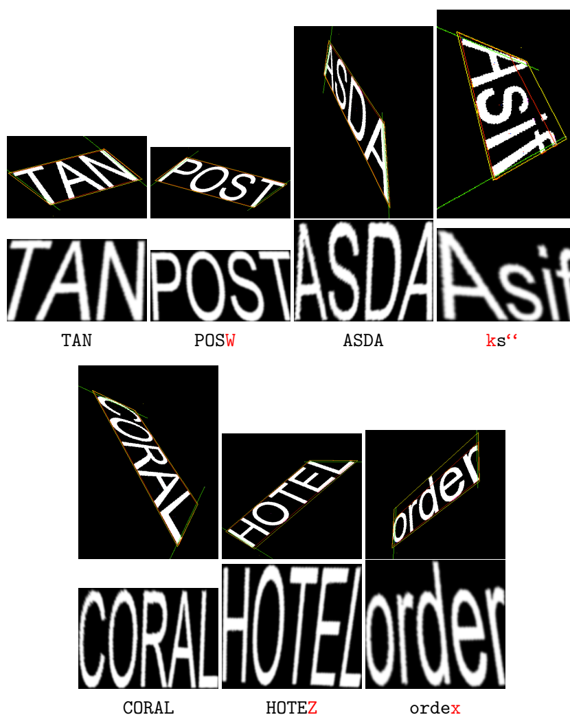
Fig. 16: Success and failures (in red) of OCR transcription of text strings containing extremity characters “A”, “T”, “L” and/or “r”: original image (top), text rectification result (middle) and OCR transcription using Tesseract (bottom).
