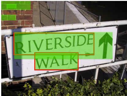
Fig. 5.14: GT (red rectangles) and detection (filled green rectangles) examples and their corresponding coverage/accuracy histograms and R_G/P_G scores.
