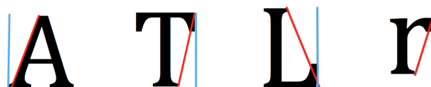
Fig. 15: Left and right bounding lines for capital letters “A”, “T”, “L” and small character “r”: incorrect approximation (red) versus correct approximation (blue).
