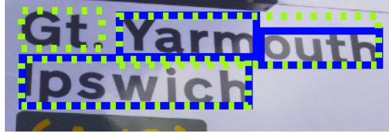
Fig. 3.9: Example of a one-to-many case (“Yarmouth” word detected two times): one text box in \mathcal{G} (dashed green) is matched to multiple boxes in \mathcal{D} (blue).
