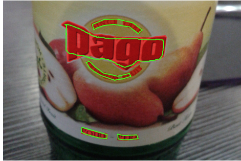
Fig. 3.22: Example of a mask detection: GT objects are shown in plain red masks and detections with green contour line.
