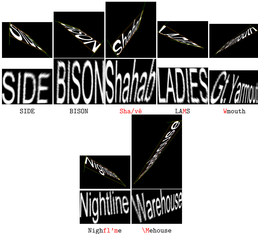
Fig. 20: Rectification result of challenging unreadable texts: original image (top), text rectification result (middle) and OCR transcription using Tesseract (bottom).
