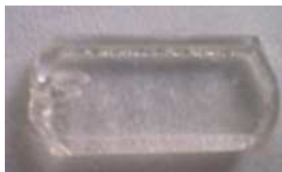
Figure I.14 : Monocristal de quartz contenant 1% de SnO 2 20
