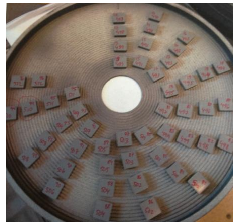
Figure 43: A tray of samples after sintering.
