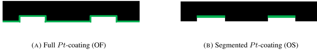
FIGURE 6.5: Studied Pt -coatings for the channel with obstacles. The green segments highlight the edges covered with Pt .
