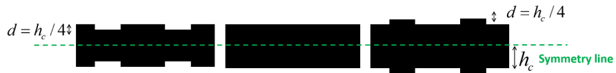
FIGURE 6.4: Reduction and increase of the planar-walls channel section by the respective introduction of obstacles and cavities. Middle : planar-wall channel, left: obstacles, right: cavities
