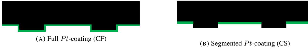
FIGURE 6.6: Studied Pt -coatings for the channel with cavities: The green segments highlight the edges covered with Pt .
