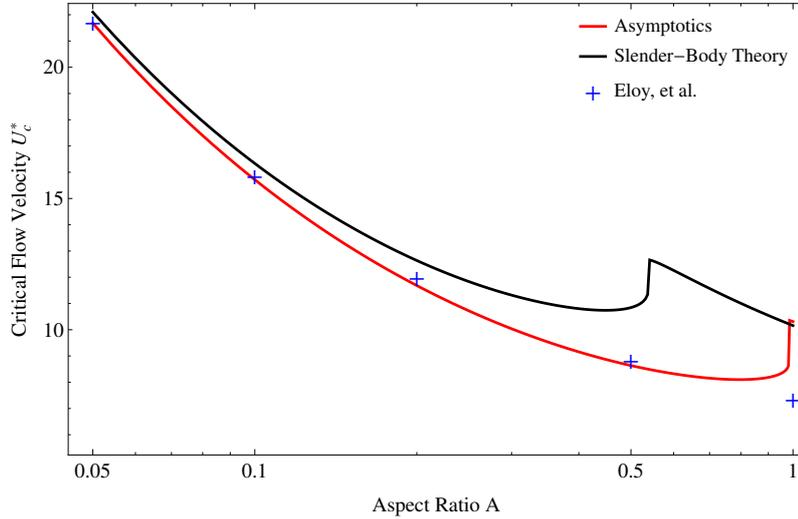
Figure 4.4 – Critical flow velocity as a function of aspect ratio  $A$  for a clamped free plate with mass ratio  $M^* = 1$ . Crosses are the results from Eloy et al. [27]. The black curve and the red one are the results derived from Slender body theory and modified asymptotic solution by acceleration potential, respectively.
