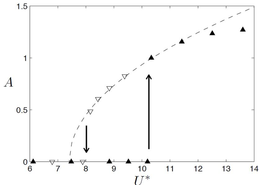
Figure 1.3 – Mode amplitude  $A$  (measured in arbitrary units) as a function of the reduced velocity. Amplitude is plotted as filled triangles when velocity is increased and open triangles when it is decreased. The aspect ratio is  $H^* = 1$  and the mass ratio is  $M^* = 0.6$ . The instability exhibits a strong hysteresis with  $U_c^* = 10.3$  and  $U_d^* = 8$ . Results from Eloy [25]
