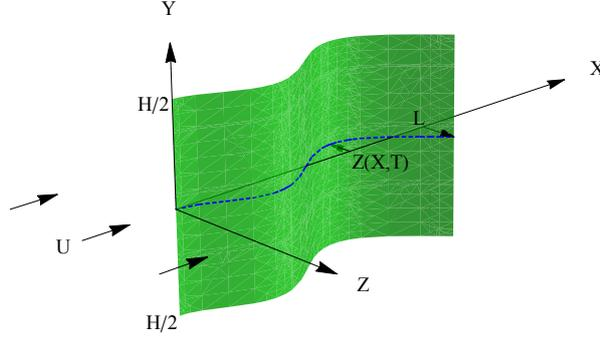
Figure 4.1 – Schematic of a plate with two-dimensional deflection  $Z(X, T)$  submerged in an axial flow of velocity  $U$ .
