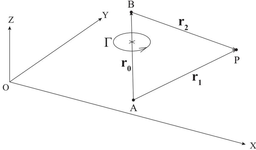
Figure 2.3 – The velocity induced by a three-dimensional, straight vortex segment.
