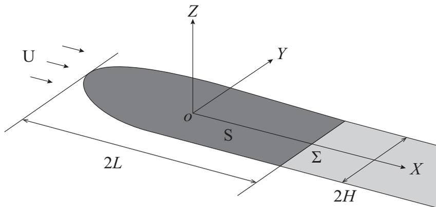
Figure 3.1 – Schematic of a lifting surface problem.
