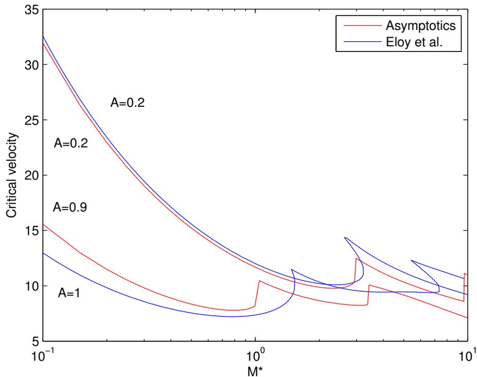
Figure 4.5 – Critical flow velocity as a function of mass ratio  $M^*$  for a clamped free plate with different aspect ratios. The red curves are the results obtained with modified asymptotic solution by acceleration potential, while the blue ones are the results of Eloy et al. [27].
