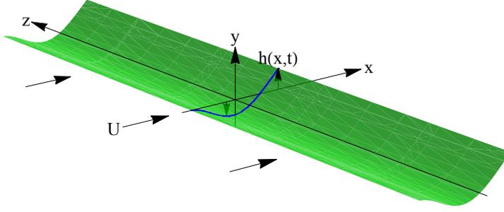
Figure 1.8 – Schematic of 2D unsteady airfoil theory.
