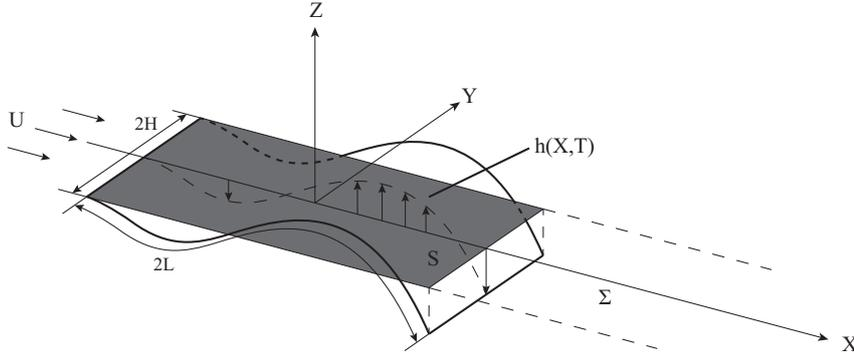
Figure 1.9 – Schematic of the lifting surface problem.
