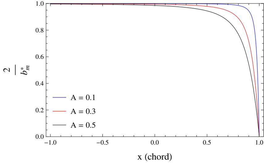
Figure 3.12 – The modified factor  $2/b^*$  as a function of chordwise coordinate for various aspect ratio.
