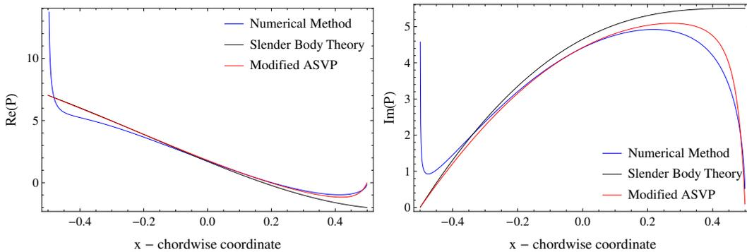
Figure 3.7 – Real and imaginary parts of the force per unit chord length,  $A = 0.3$ ,  $k = 0.5$ , first beam eigenmode.
