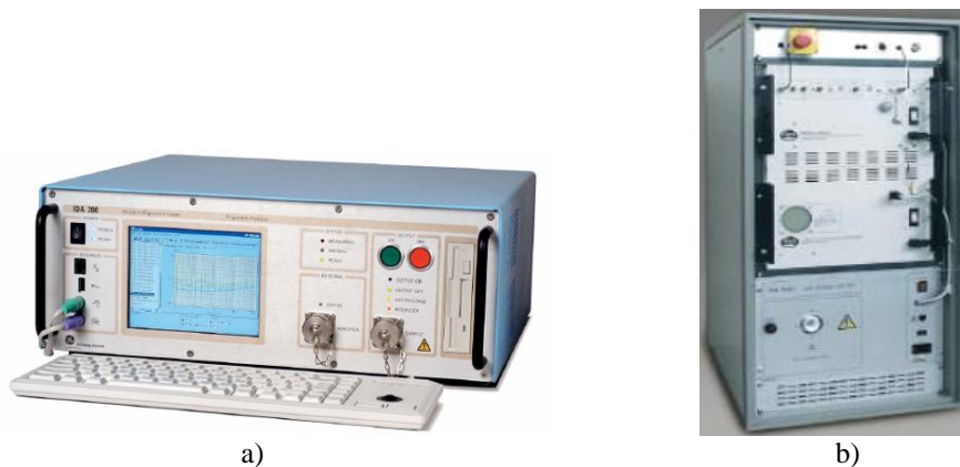
Figure 29 : Dispositif Programma IDA200: a) IDA200, b) IDA200 HVU (High Voltage Unit).
