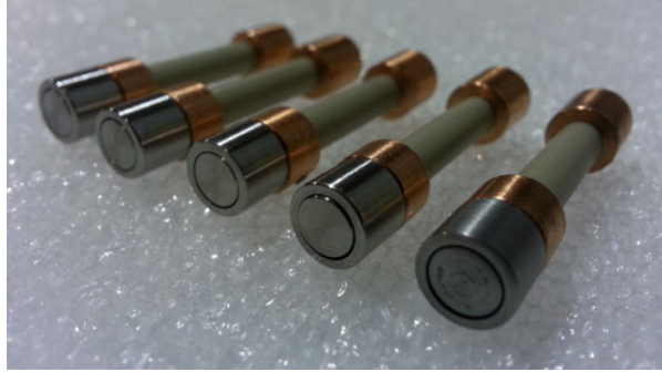
Figure 4.12: The five Faraday probes that have been characterized in the plume of the PPI-Mag. Four are made of stainless steel. A fifth probe is made of molybdenum (far-right) to evaluate the influence of the probe material on the current that is measured. The guard ring can be removed if necessary, in order to obtain a nude Faraday probe.
