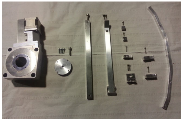
Figure 4.15: Parts that compose the rotating arm. From left to right: rotation stage, mechanical interface, horizontal and angled beams, beam/arch interface and probe holders, arch.
