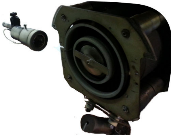
Figure 9: Photograph of the SPT100-ML Hall thruster. The magnetic circuit and outer ceramic ring have been machined to allow LIF measurements in the discharge channel. The fluorescence collection optical assembly is shown, and is aligned on the slit to pinpoint the channel axis.
