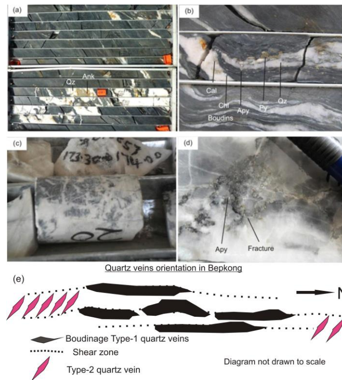
Fig. 5.8. Photograph of drill core showing the various characteristic of Type-1 quartz veins observed within the Bepkong deposit (a) Drill core showing 3 m of crystalline Type-1 quartz veins within the dilatational zone of the anastomosing D_{B1} shear zone. Within these veins are ankerite (Ank) and quartz (Qz) (b) Boudinage Type-1 quartz veins folded by the F_{B3} fold within the Bepkong deposit. Pyrite (Py), calcite (Cal), Chlorite (Chl) and the arsenopyrite (Apy) are at the selvages of the veins. (c) Veins exhibiting breccia. The breccias are mainly inclusions from the country rock and give an indication of a brief change in the fluid temperature and pressure in an overall ductile regime within the deposit (d) Type-1 Quartz veins showing fractures. The fractures have been filled with arsenopyrite and secondary minerals such as chlorite, calcite, and sericite. (e) Schematic diagram of quartz vein orientation in the Bepkong deposit.
