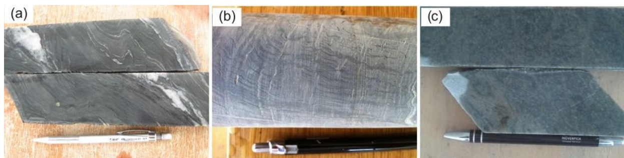
Fig. 5.2. Drill core images of rocks in the Bepkong deposit (a) Fresh deformed shale in the Bepkong deposit (b) Volcaniclastic rock in the Bepkong deposit exhibiting some spaced cleavages (c) highly sheared microdiorite rock.
