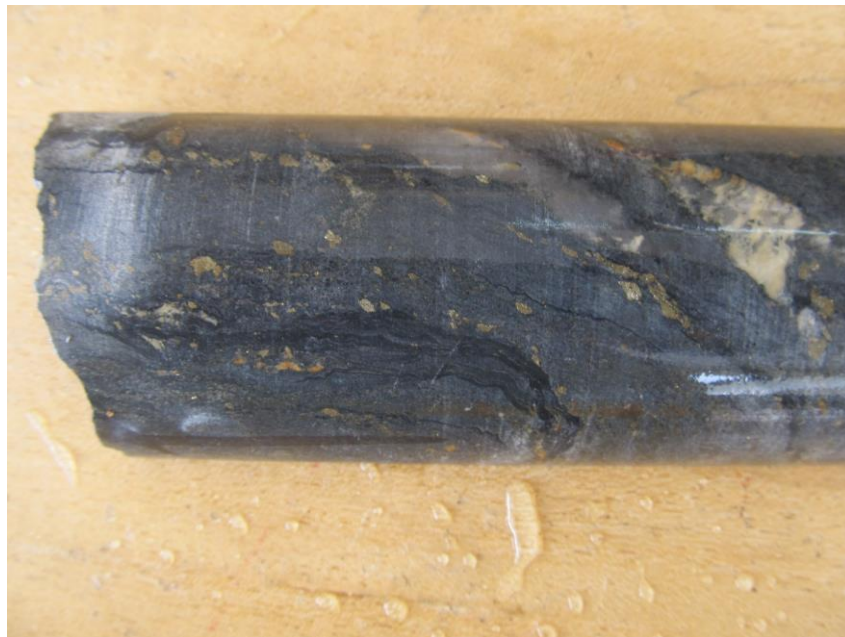
Fig 6.3. Borehole showing mylonised granodiorite with the early stage pyrite deformed showing a sigmoidal features.
