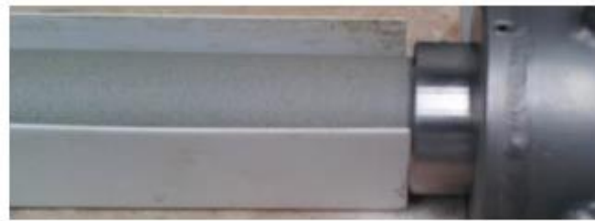
Figure. 5.13. Surface of the extruded cement mortar
