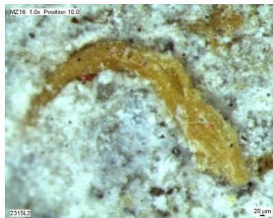
Figure 6.23. Micrograph composite after failure compression of static loading, for broken fiber.
