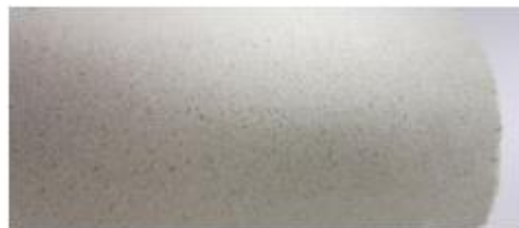
Figure. 5.9. Surface of the extruded mortar type C1
