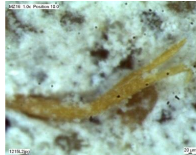
Figure 6.23. Micrograph composite after failure compression of static loading, for broken fiber.
