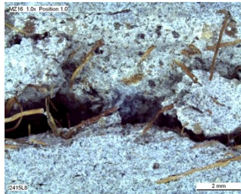
Figure 6.22. Micrograph coir fiber reinforced cementitious composites, after failure compression of static loading.
