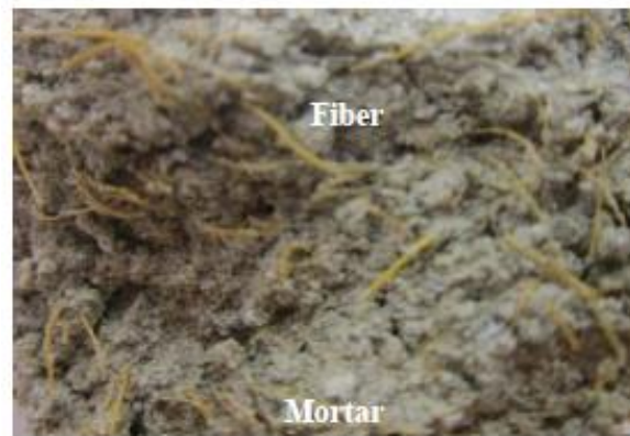
Figure. 5.14. Morphology of fiber-reinforced cementitious composites after mixing.
