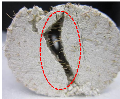
Figure. 6.27. Coir fiber orientation longitudinal direction of extrusion of coir fiber cement clay mortar composites.
