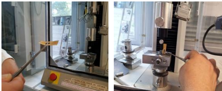
Figure.3.9. Preparation of specimen for the tensile test
