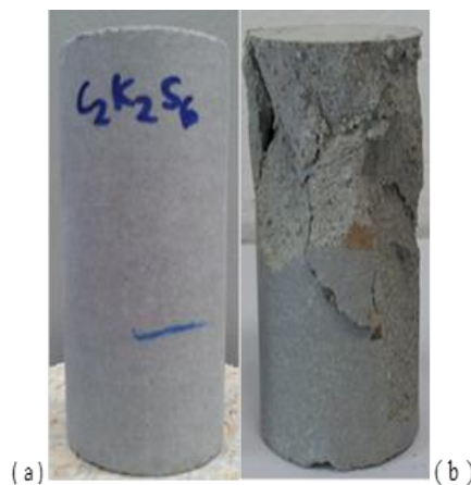
Figure 6.19. Typical compression failure modes of extruded cement mortar type C2 non-fiber: (a) plain mortar; (b) after static loading.
