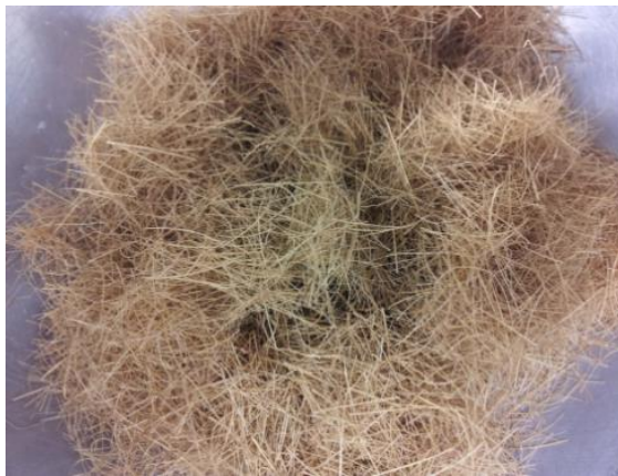
Figure 3.16. Chopped Coir Fibers
