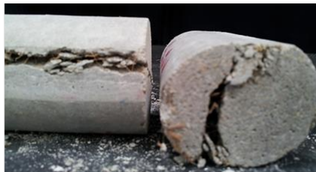
Figure 6.25. Typical tension failure modes under static loading of coir fiber cementitious composite.
