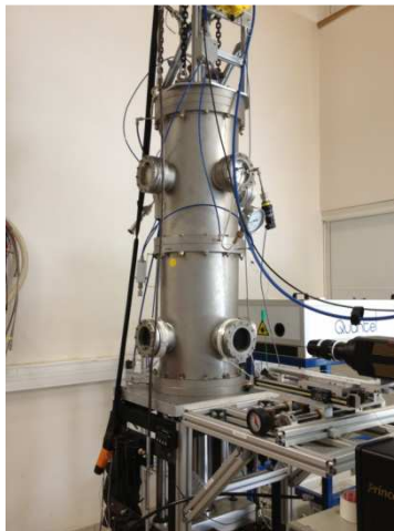
Figure 15: Chambre de combustion
