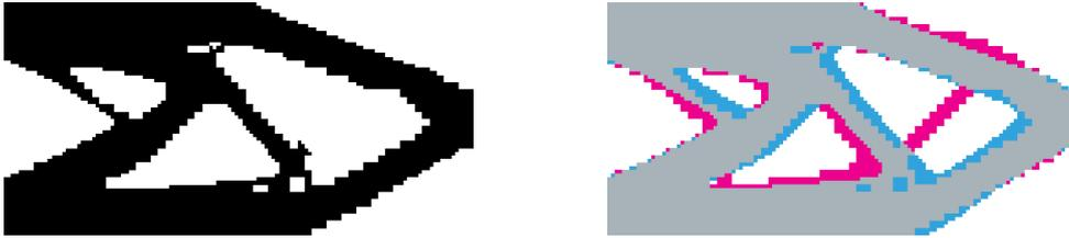
Fig. 4.10 Detailed design comparison for  $c_{er} = 0.01$  for the different mesh densities; *left*: common region; *right*: additional material for  $n_y = 32$  (magenta) and  $n_y = 64$  (blue); tip deflection  $\bar{u} = 10$  mm
