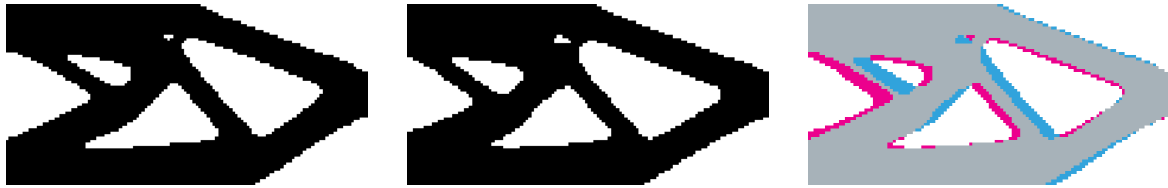
Fig. 4.13 Comparison of the two designs for the finer mesh; left to right : final design for \bar{u} = 10\text{mm} , \bar{u} = 20\text{mm} , comparison (gray: common, blue: additional for 10 mm, magenta: additional for 20 mm)
