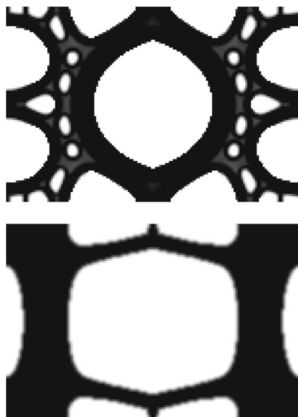
Fig. 11 Materials with maximized bulk moduli obtained using sensitivity filtering ( top , c = -0.6730 , iteration 345) and density filtering ( bottom , c = -0.6317 , iteration 349) with penalty factor p = 5 and filter radius r = 2
