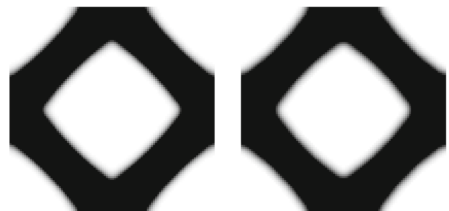
Fig. 12 Materials with maximized shear moduli obtained using sensitivity filtering ( left , c = -0.1256 , iteration 12) and density filtering ( right , c = -0.1213 , iteration 72) with penalty factor p = 3 and filter radius r = 5
