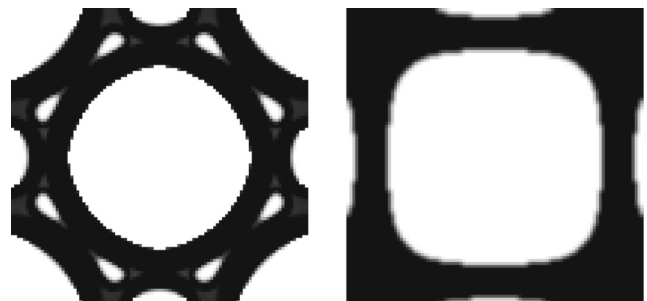
Fig. 10 Materials with maximized bulk moduli obtained using sensitivity filtering (left, c = -0.6793 , iteration 183) and density filtering (right, c = -0.6540 , iteration 129) with penalty factor p = 5 and filter radius r = 2
