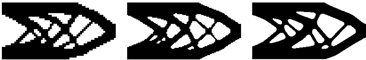
Fig. 4.5 Design solutions for linear elasticity for the three mesh resolutions 64 \times 32 , 128 \times 64 and 256 \times 128 elements (left to right; macroscopic volume fraction of solid material 60%)
