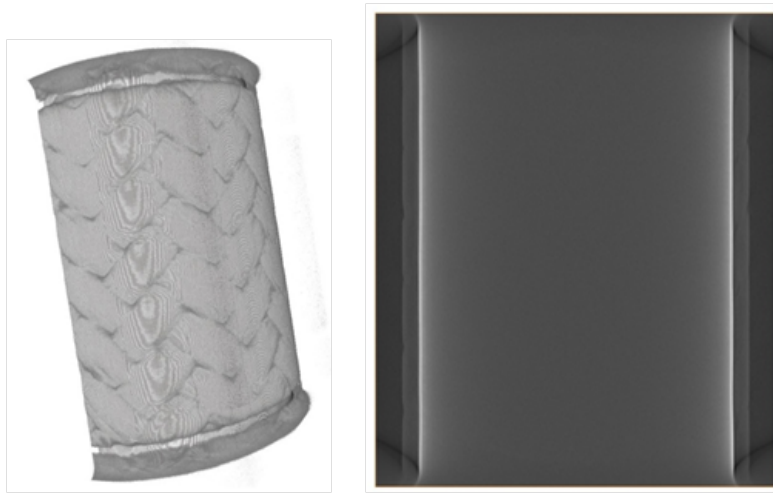
FIGURE 2.41 – Tomographies X de la gaine sandwich
