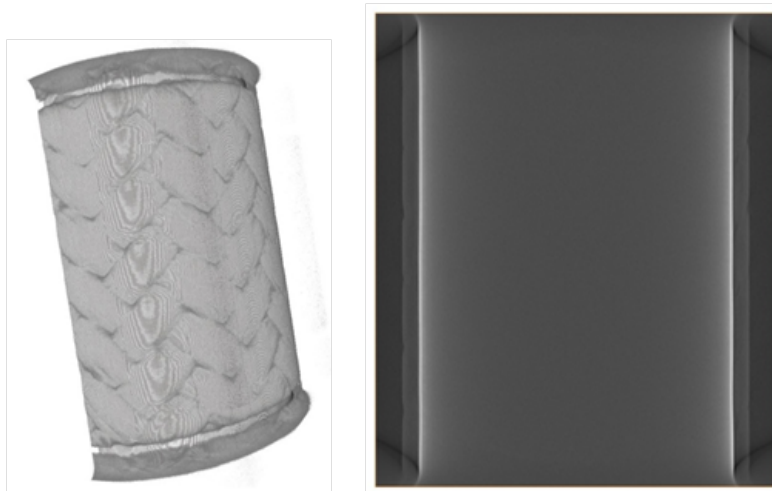
FIGURE 2.41 – Tomographies X de la gaine sandwich
