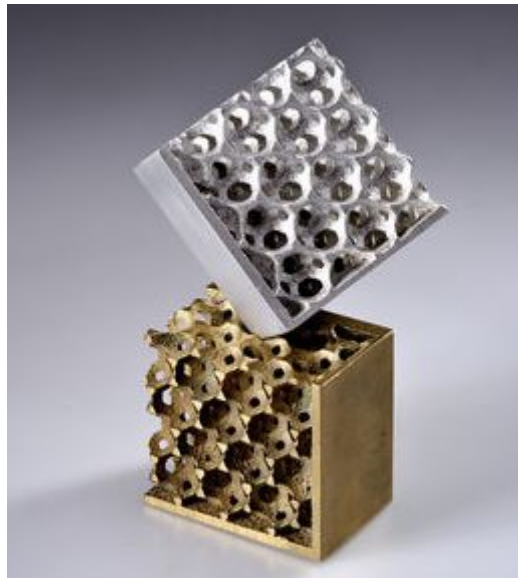
Figure 1.2: Homogeneous metallic foams d_p = 14 \text{ mm} , top: Aluminium, bottom: Copper
