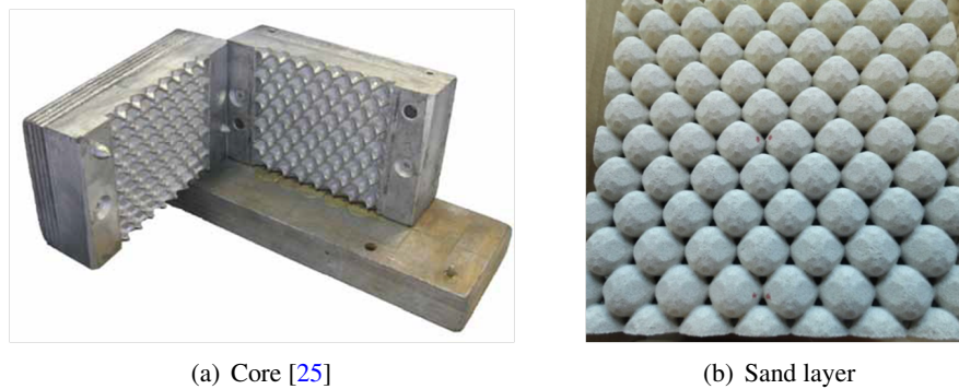
Figure 4.35: Core used to create the sand layers formed of spherical cells
