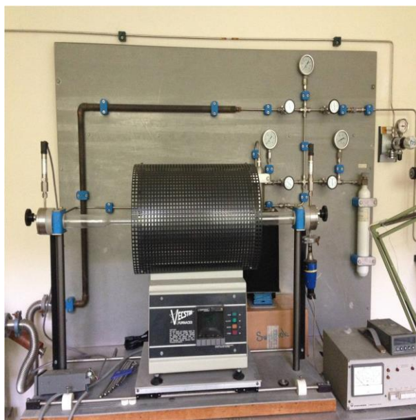
Figure 3.4 Image of oxidation furnace with ^{18}\text{O}_2 in SP2M/ICMMO
