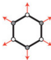
Figure 4 : Atom displacements in the breathing mode leading to the D band.
