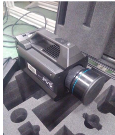
Figure 2.15 - Caméra infrarouge FLIR X6540sc.
