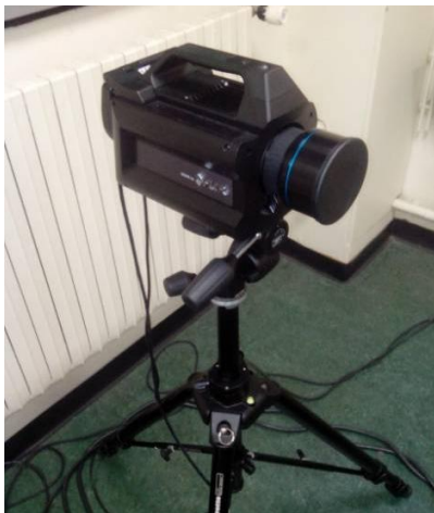
Figure 2.15 - Caméra infrarouge FLIR X6540sc.
