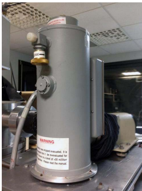
Figure 2-20 CCD camera with cooling system from Princeton Instruments (LN / CCD-1100-PB).
