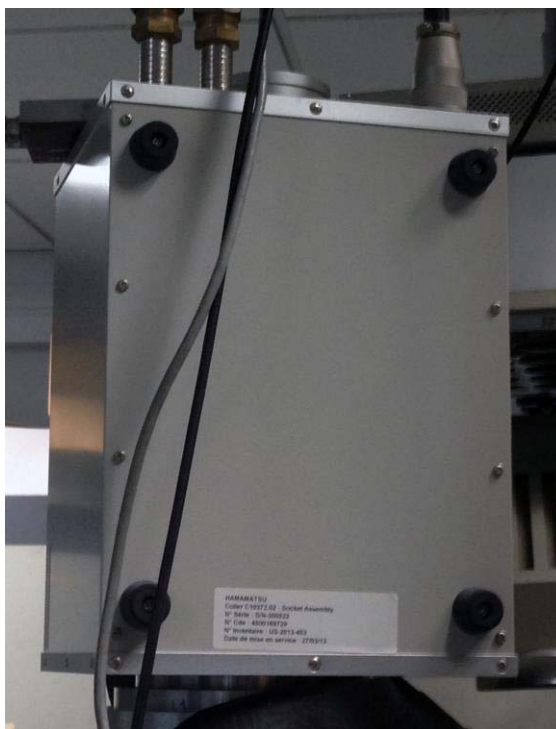
Figure 2-19 The photomultiplier with cooling system of Hamamatsu R943-02.
