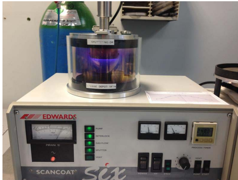
Figure 2-5 Gold metallization setup, Scancoat 6 from Edwards.
