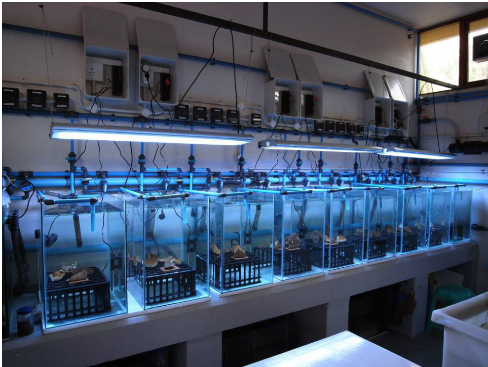
Figure 15: Experimental set-up of inoculation trials showing the nine 100 l tanks individually supplied with oligotrophic seawater and exposed to constant, artificial light.
