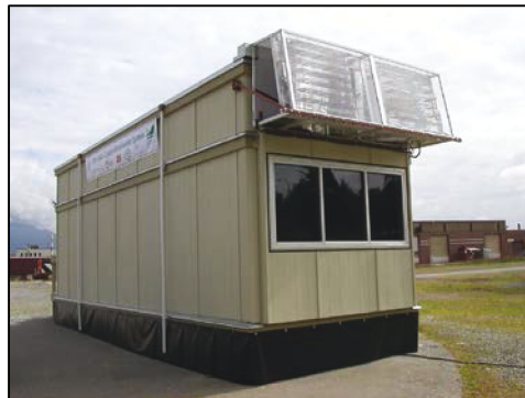
Figure 7 : Solar Canopy Illumination System (Rosemann, Mossman, and Whitehead 2008)
