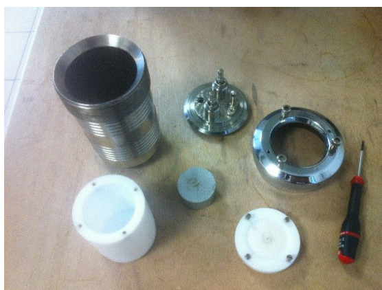
Figure 1.3: Teflon-lined stainless steel autoclave built for MIL-101(Cr) synthesis
