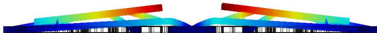
Figure 145: Sense mode (Dynamic acceleration) obtained by FEM for a coupled accelerometer-gyroscope structure (20.0 kHz)
