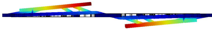
Figure 144: Sense mode (Coriolis force) obtained by FEM for a coupled accelerometer-gyroscope structure (20.5 kHz)
