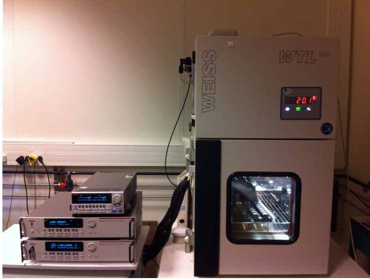
Figure 20: Experimental setup using temperature controlled chamber
