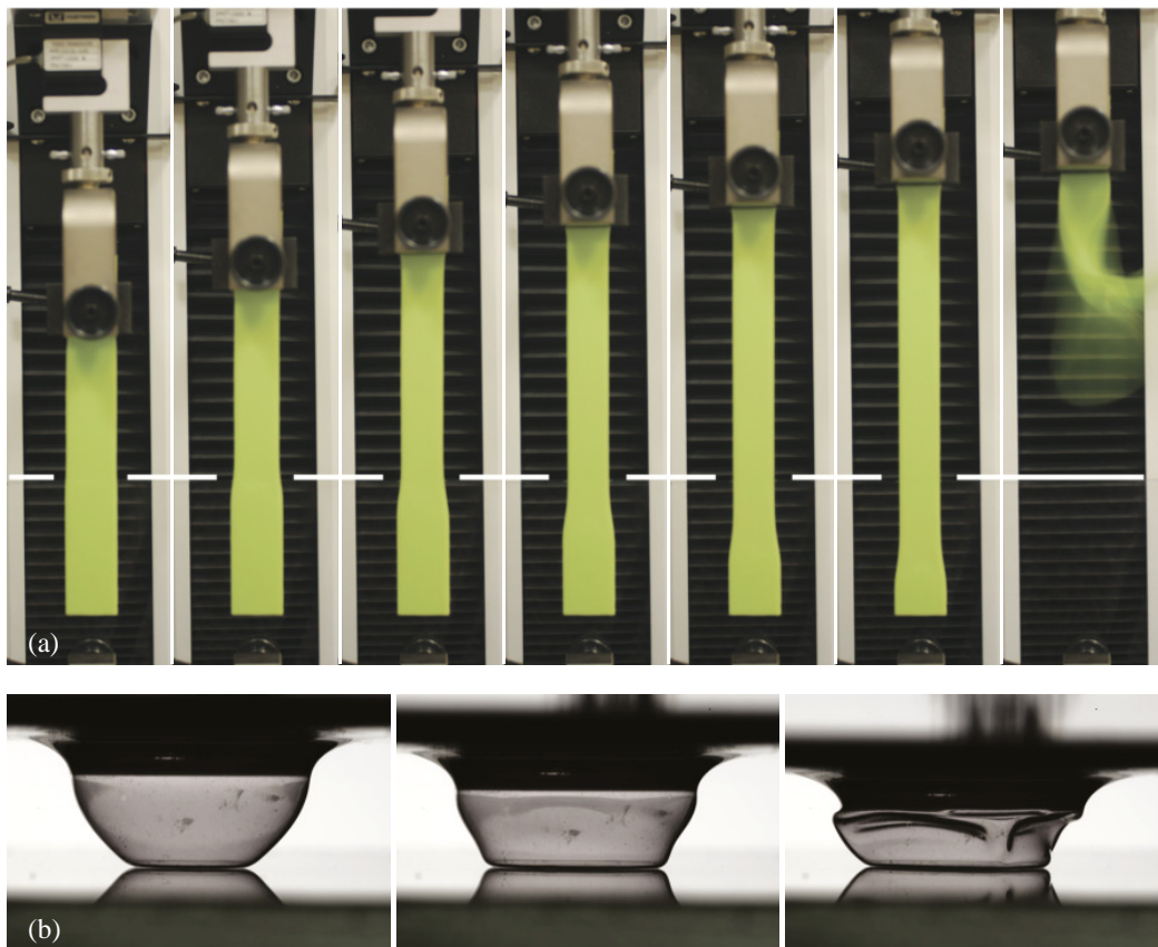
Figure 1.3.: Configurations investigated in the present thesis: (a) peeling of an elastomeric tape adhering on a smooth tape, (b) punch test with a highly compliant shell.
