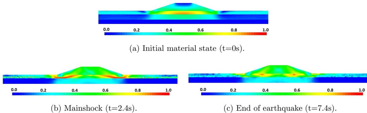
Figure 6.12: Typical dynamic response (irsn168 motion): Contours of residual strength,  $r_k$ .
