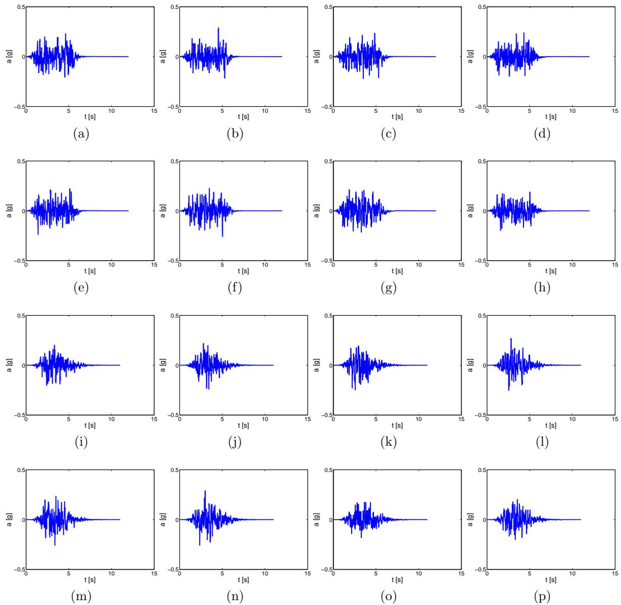
Figure C.15: Accelerograms of synthetic earthquakes generated in Code\_Aster .
