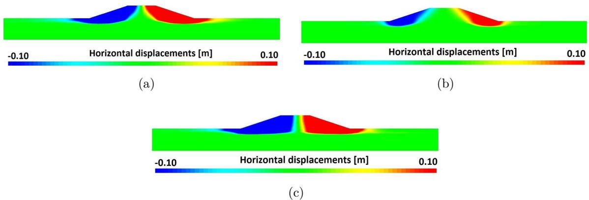
Figure 6.39: Horizontal displacements at the end of the ground motion: a) Low (Rb 5), b) Moderate (irsn168), c) Strong (Ra 9).
