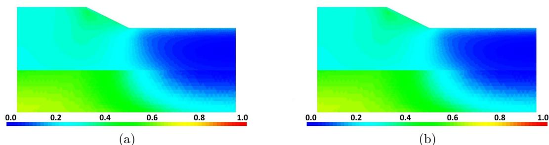
Figure 5.26: Contours of residual strength,  $r_k$ , before the ground motion (LMS model): a) Fully drained effective stress simulation, b) Coupled effective stress simulation.
