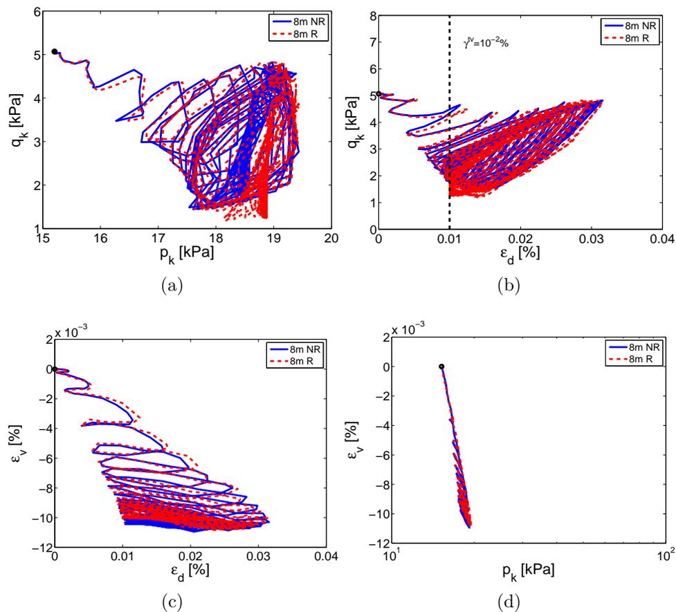
Figure G.17: Mechanical behavior with zero shear-induced volumetric deformations (8m from base): a)  $p_k$ - $q_k$ , b)  $q_k$ - $\varepsilon_d$ , c)  $\varepsilon_v$ - $\varepsilon_d$ , d)  $p_k$ - $\varepsilon_v$ .
