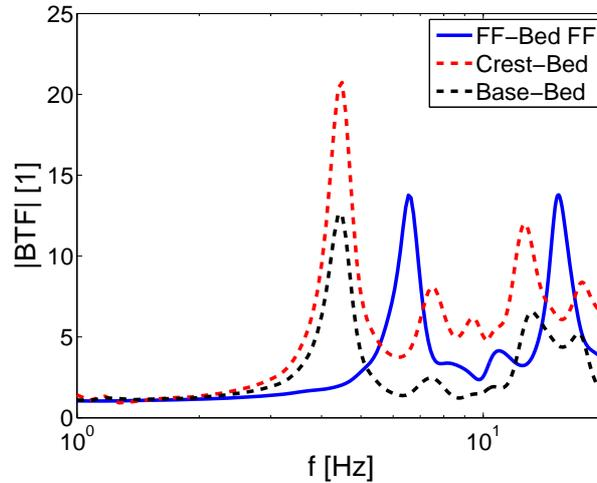
Figure 6.4: Borehole Transfer Function of levee - foundation system.
