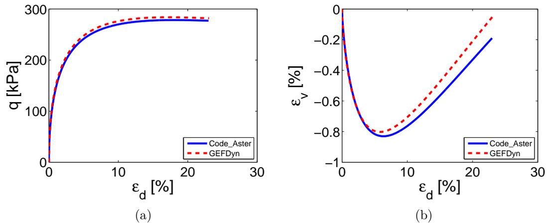
Figure D.1: Comparison of soil response of one material point with the ECP constitutive model ( $p_0=100\text{kPa}$ ,  $K_0=1.0$ ) under biaxial drained test: a)  $q - \varepsilon_d$ , b)  $\varepsilon_d - \varepsilon_v$ .
