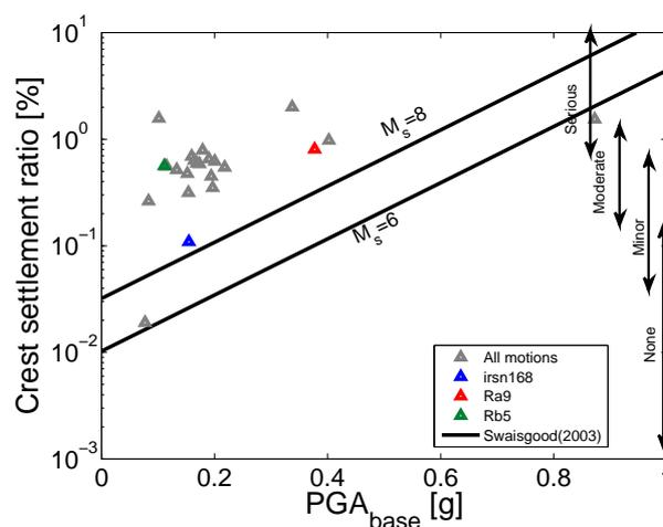
Figure 6.37: Comparison of the crest settlement ratio of the FE model: in grey all motions and in color the selected motions.
