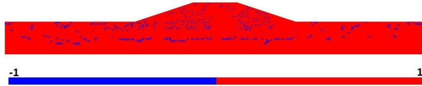
Figure 6.16: Liquefiable layer in depth (Ra9 motion): Contours of second order work at the end of earthquake.
