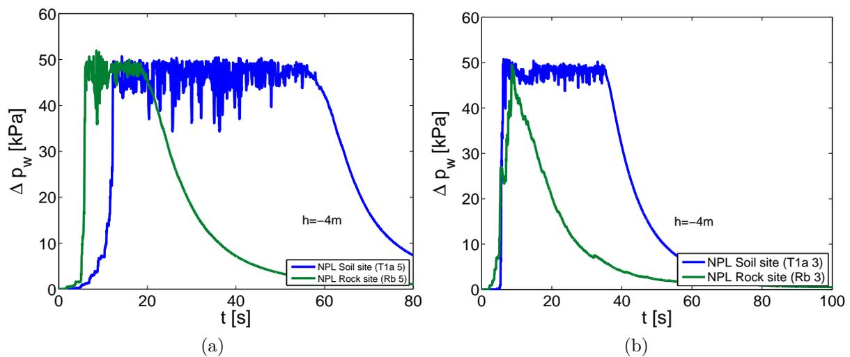
Figure 3.29: Evolution of pore water pressure (at  $h=-4\text{m}$  from the surface): a) Comparison NPL soil site motion (T1a 5) - NPL rock site motion (Rb 5), b) Comparison NPL soil site motion (T1a 3) - NPL rock site motion (Rb 3).
