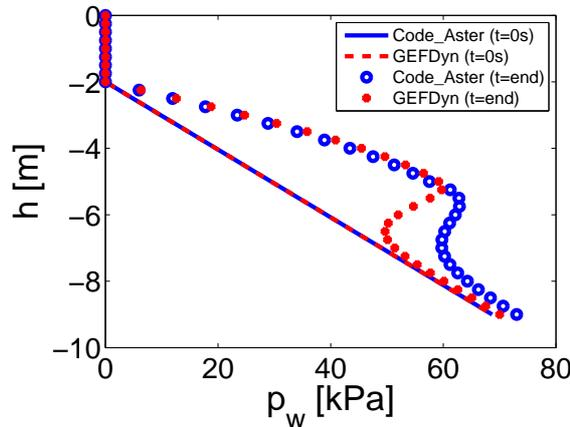
Figure 3.7: Comparison Code\_Aster -GEFDyn: Profile of pore water pressure ( $p_w$ ) along the column's lateral surface.
