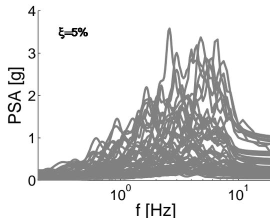
Figure 3.36: Acceleration spectra of input motions ( $\xi=5\%$ ).
