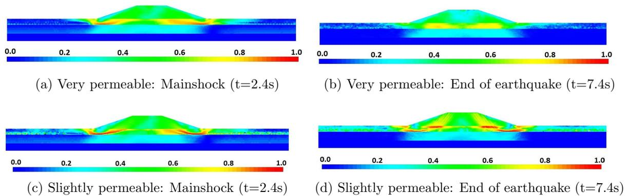
Figure 6.27: Influence of soil's permeability (irsn168): Contours of residual strength,  $r_k$ . a) Initial material state identical for all models, b,c) Very permeable, d,e) Permeable, f,g) Slightly permeable.
