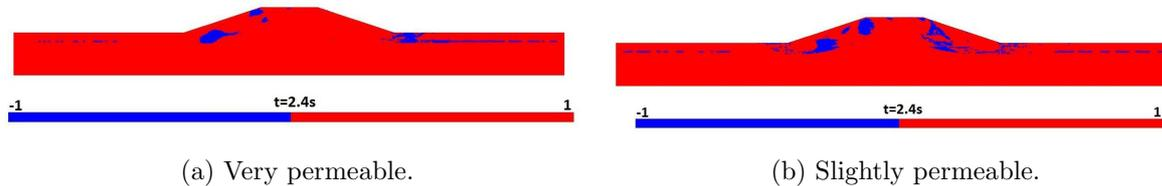
Figure 6.25: Influence of soil's permeability (irsn168): Contours of second order work during the mainshock ( $t=2.4s$ ).
