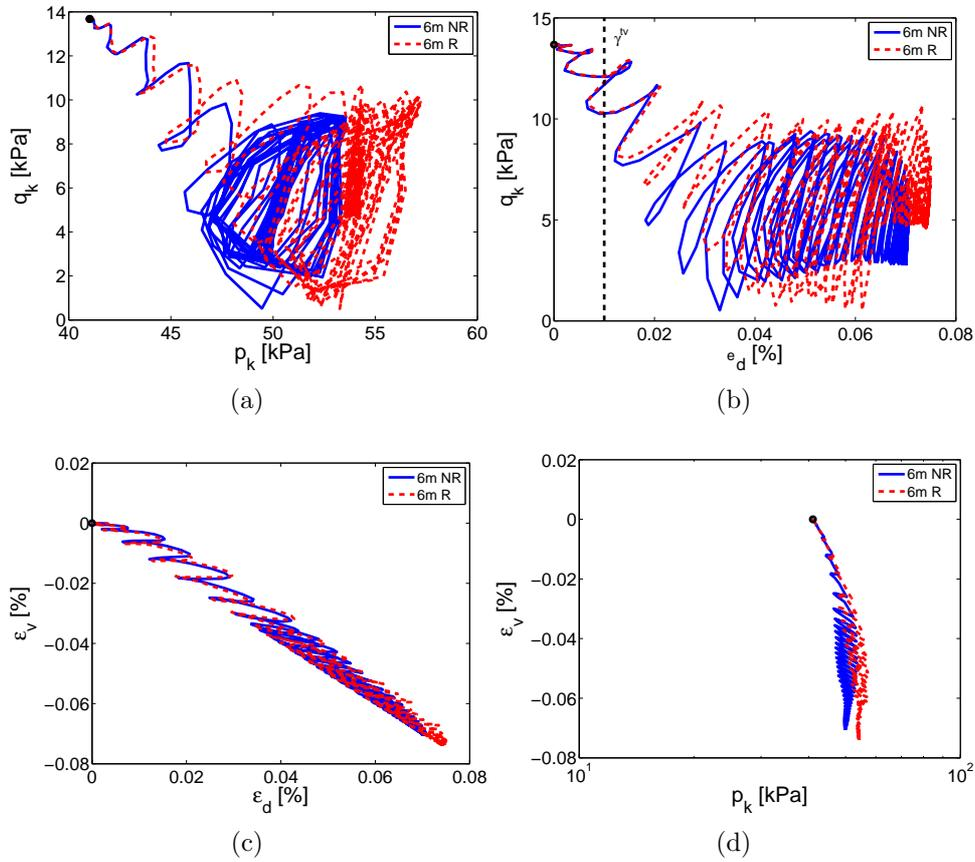
Figure G.9: Mechanical behavior (6m from base): a)  $p_k$ - $q_k$ , b)  $q_k$ - $\epsilon_d$ , c)  $\epsilon_v$ - $\epsilon_d$ , d)  $p_k$ - $\epsilon_v$ .
