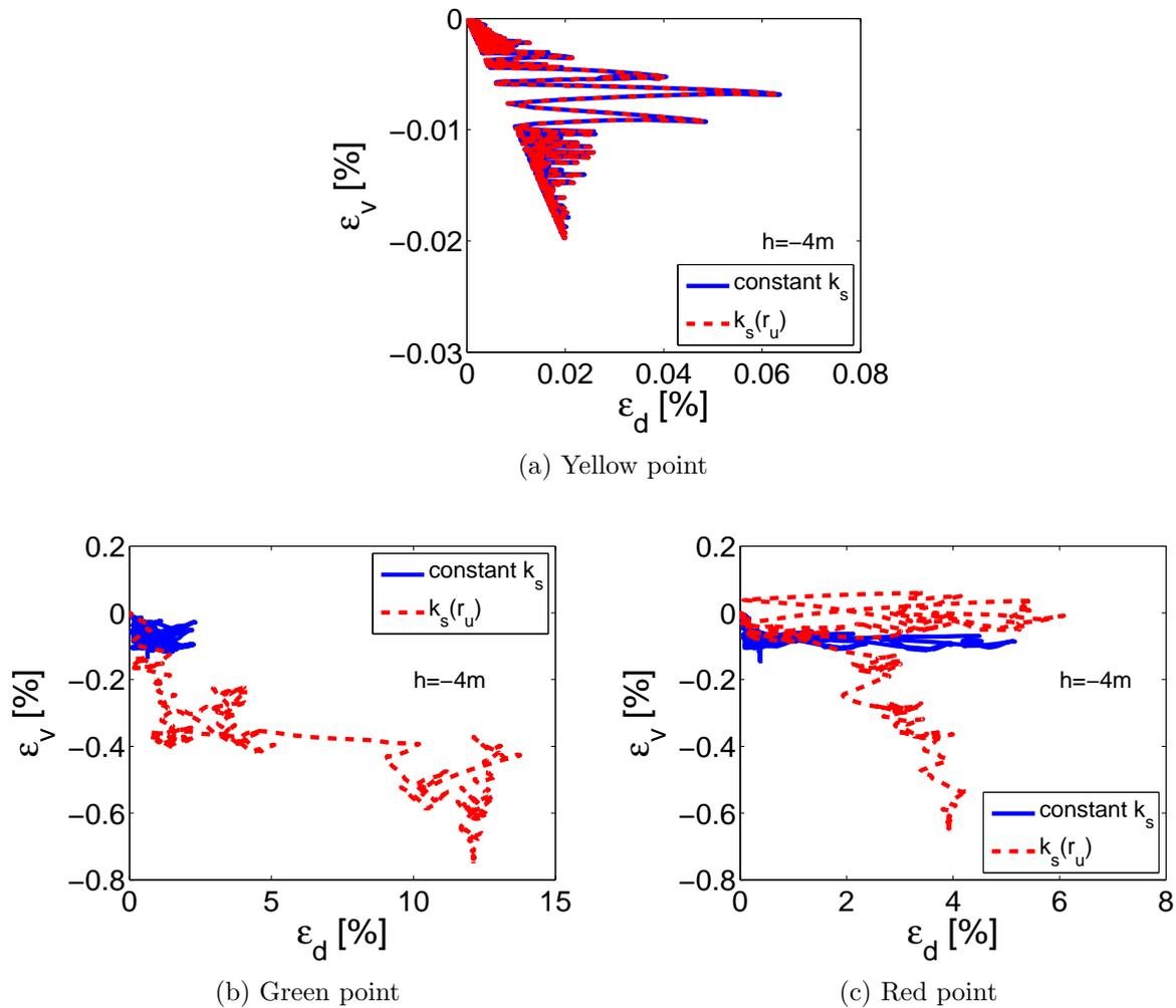
Figure 3.47: Comparison of volumetric - deviatoric deformations at  $h = -4\text{m}$  from surface.
