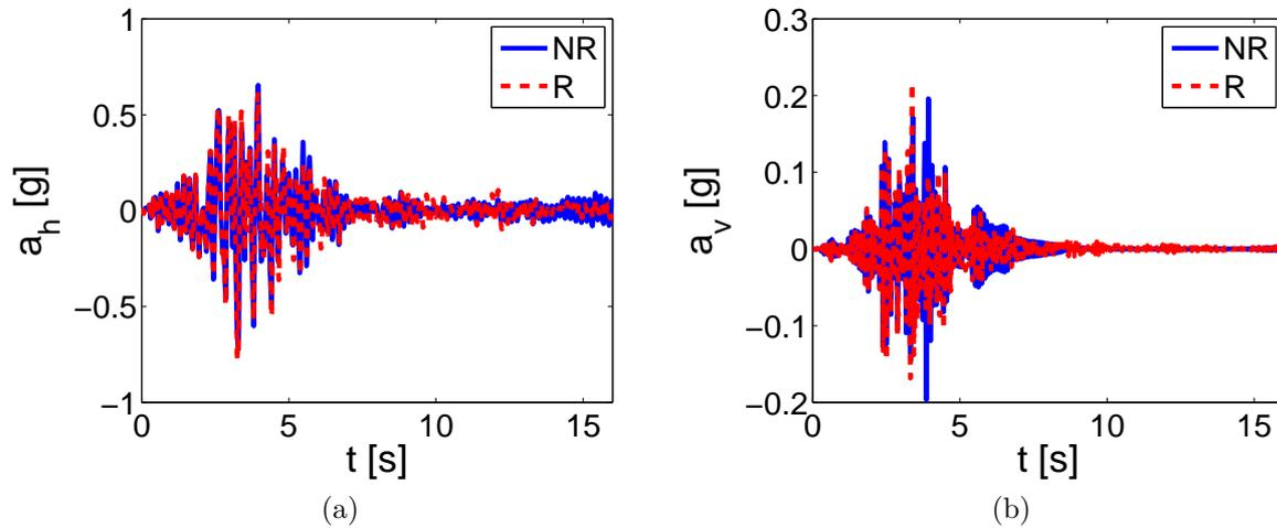
Figure 4.7: FF acceleration without and with regularization: a) Horizontal, b) Vertical-induced.
