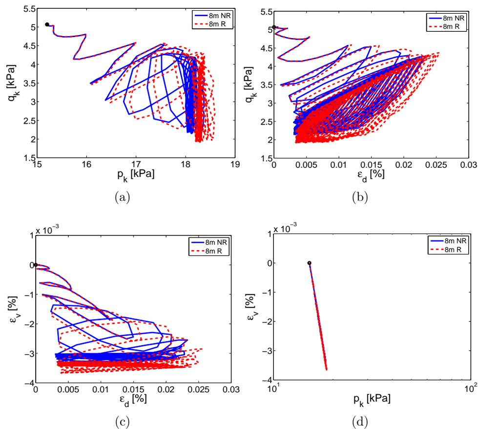
Figure G.21: Mechanical behavior with isotropic mechanism deactivated and zero shear-induced volumetric deformations (8m from base): a)  $p_k$ - $q_k$ , b)  $q_k$ - $\epsilon_d$ , c)  $\epsilon_v$ - $\epsilon_d$ , d)  $p_k$ - $\epsilon_v$ .
