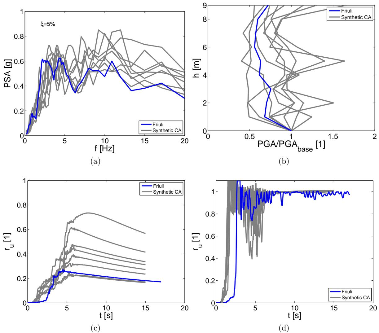
Figure 6.48: Comparison of results obtained by synthetic motions and Friuli: a) Response spectrum PSA at crest as function of frequency, b) Profile of normalized PGA at the levee's middle cross-section, c) Evolution of excess pore water pressure ratio ( $r_u$ ) below the levee (P5), d) Evolution of excess pore water pressure ratio ( $r_u$ ) below FF (P6).
