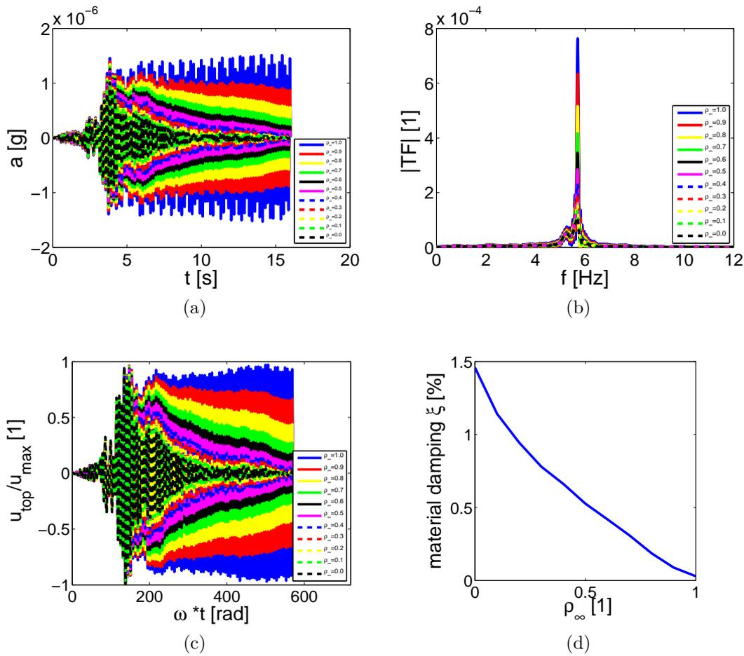
Figure A.1: Parametric analysis for different sets of Newmark parameters: a) Horizontal acceleration at the top of the column relative to the base, b) Transfer function, c)  $u_{top}/u_{max} - \omega \cdot t$ , d) Evolution of material damping as function of  $\rho_\infty$ .
