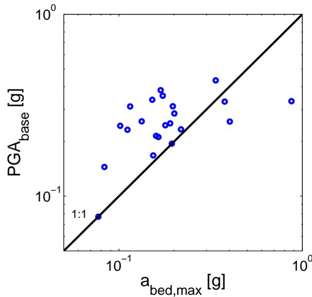
Figure 6.35: Comparison of the bedrock's to base's PGA.
