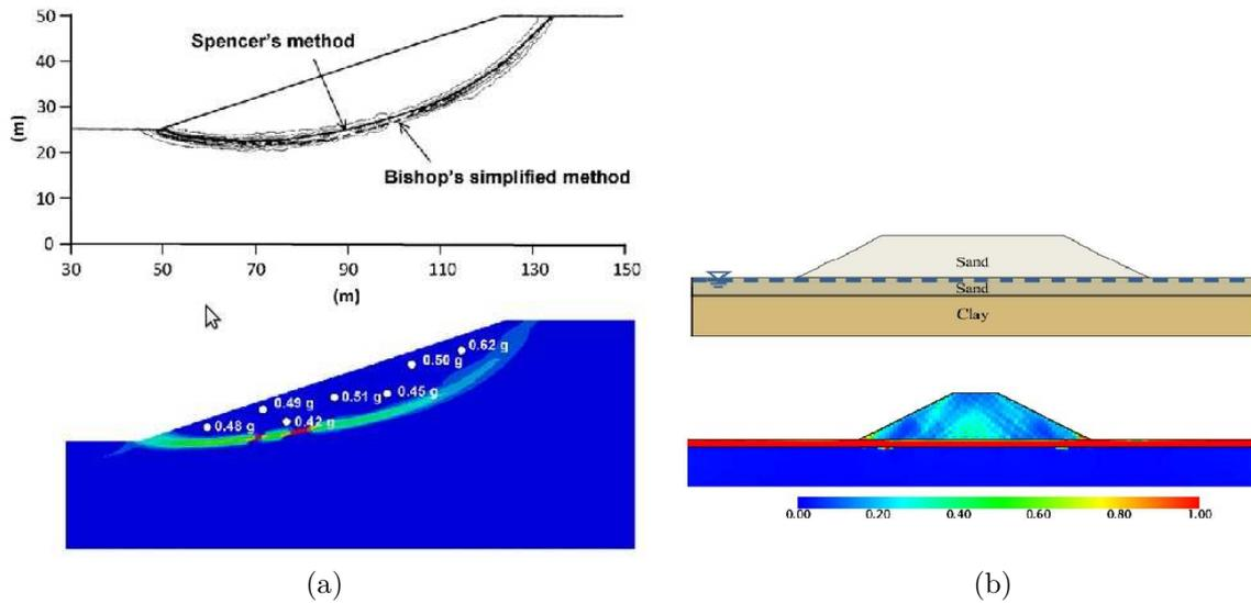
Figure 1.3: Numerical modeling of slope stability: a) FE limit analysis failure surface compared with Bishop's and Spencer's limit equilibrium methods (Kourkoulis et al., 2010), b) Numerical model and distribution of accumulated plastic deviatoric strain (Oka et al., 2012).
