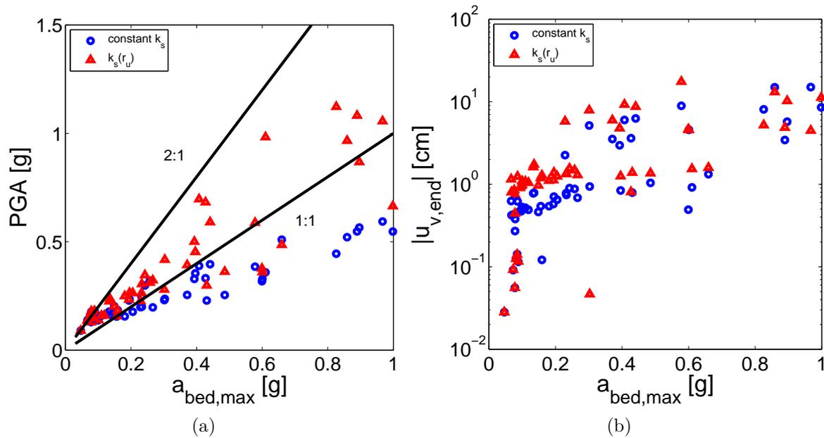
Figure E.4: Comparison in case of silty sand: a) PGA, b) Ground settlement at the end of the ground motion.
