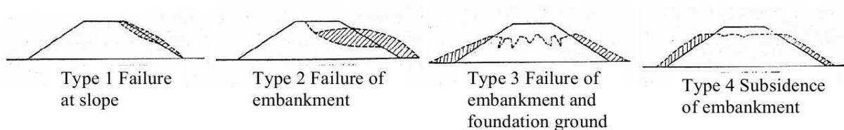
Figure 6.1: Classification of damage modes of failed dikes (Sasaki and Tamura, 2007).
