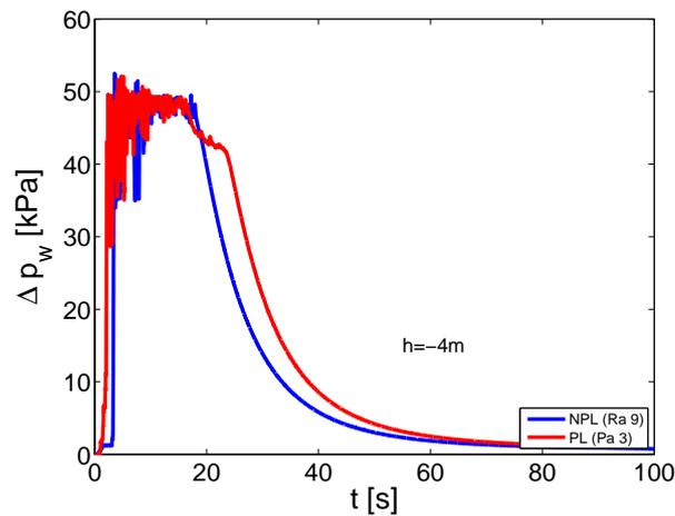
Figure 3.34: Evolution of pore water pressure (at  $h=-4m$  from the surface): Comparison NPL (Ra 9) - PL (Pa 3).
