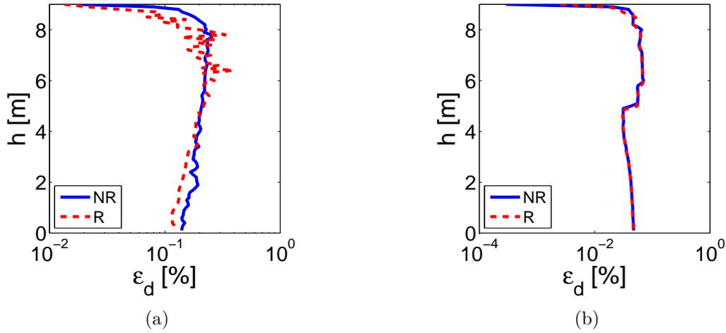
Figure 4.5: Profile of deviatoric strains  $\varepsilon_d$  at the end of the ground motion: a) Dilatancy rule activated, b) Dilatancy rule deactivated: No shear-induced volumetric strains.
