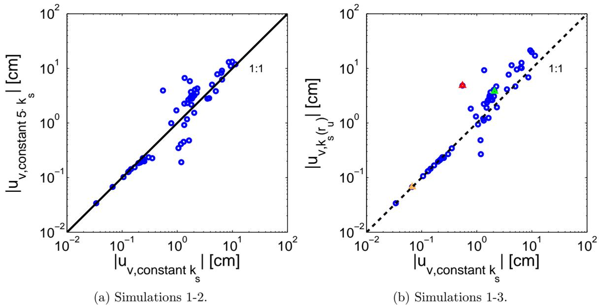
Figure 3.46: Comparison of settlement at the end of the ground motion.
