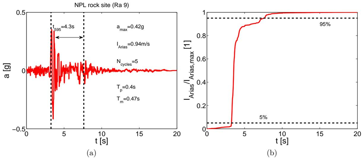
Figure 6.13: Input seismic signal (Ra9): a) Accelerogram, b) Normalized Arias intensity.
