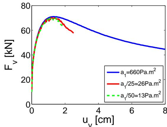
Figure F.8:  $F_v - u_v$  curve of Hostun sand (DR=88%) at confining pressure  $p_0=-100\text{kPa}$ .
