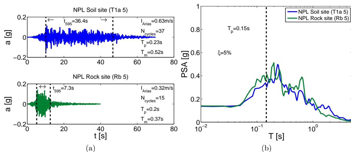
Figure 6.44: Input ground motions for comparison NPL soil site motion-NPL rock site motion: a) Accelerograms T1a 5/Rb 5, b) Acceleration response spectra ( $\xi=5\%$ ) T1a 5/Rb 5 and T1a 3/Rb 3 ( $T_p$  of levee is indicated with the dashed line).
