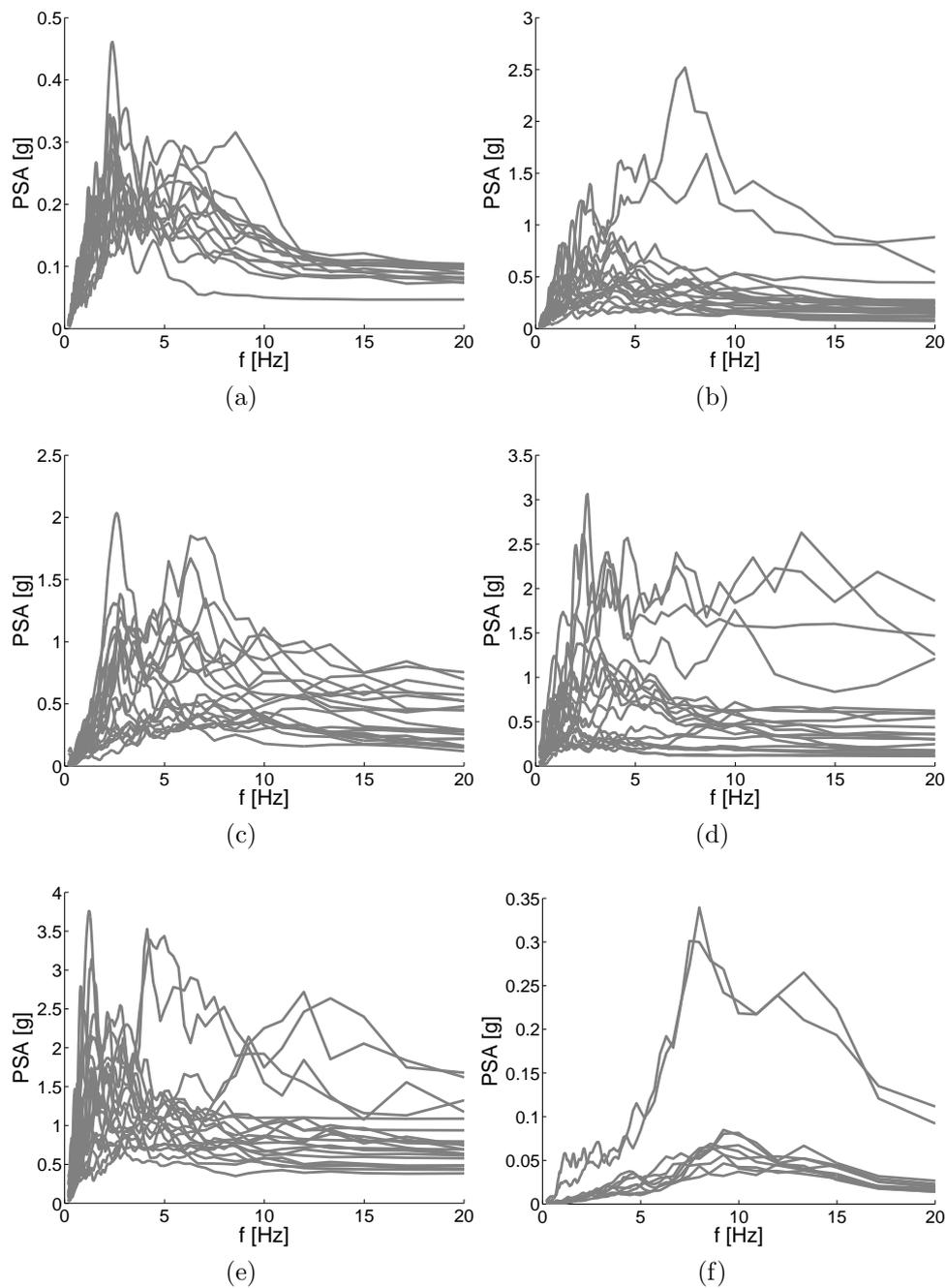
Figure C.9: Acceleration spectrum of real input seismic motions ( $\xi=5\%$ ): a) Low non pulse-like recorded on soil site, b) Moderate non pulse-like recorded on soil site, c) Non pulse-like recorded on rock site, d) Pulse-like, e) Near-Fault, f) Low from kik-Net network.
