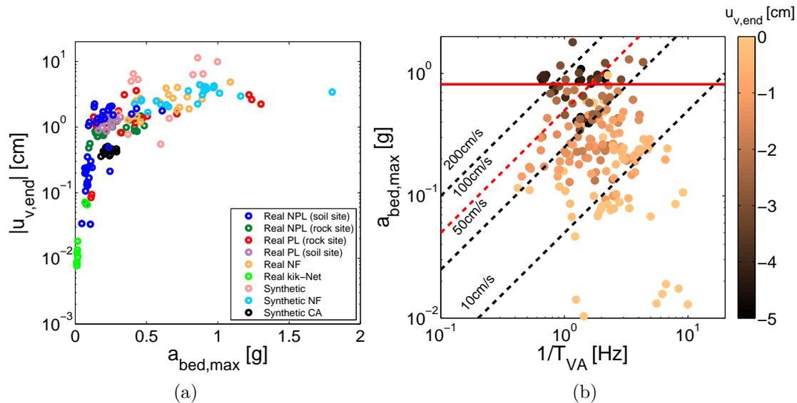
Figure 3.21: Settlement  $u_v$  at free-field classified according to: a) input signal's type as function of  $a_{bed,max}$ , b) relation between input IM:  $a_{bed,max}$  and  $T_{V,A}$ .
