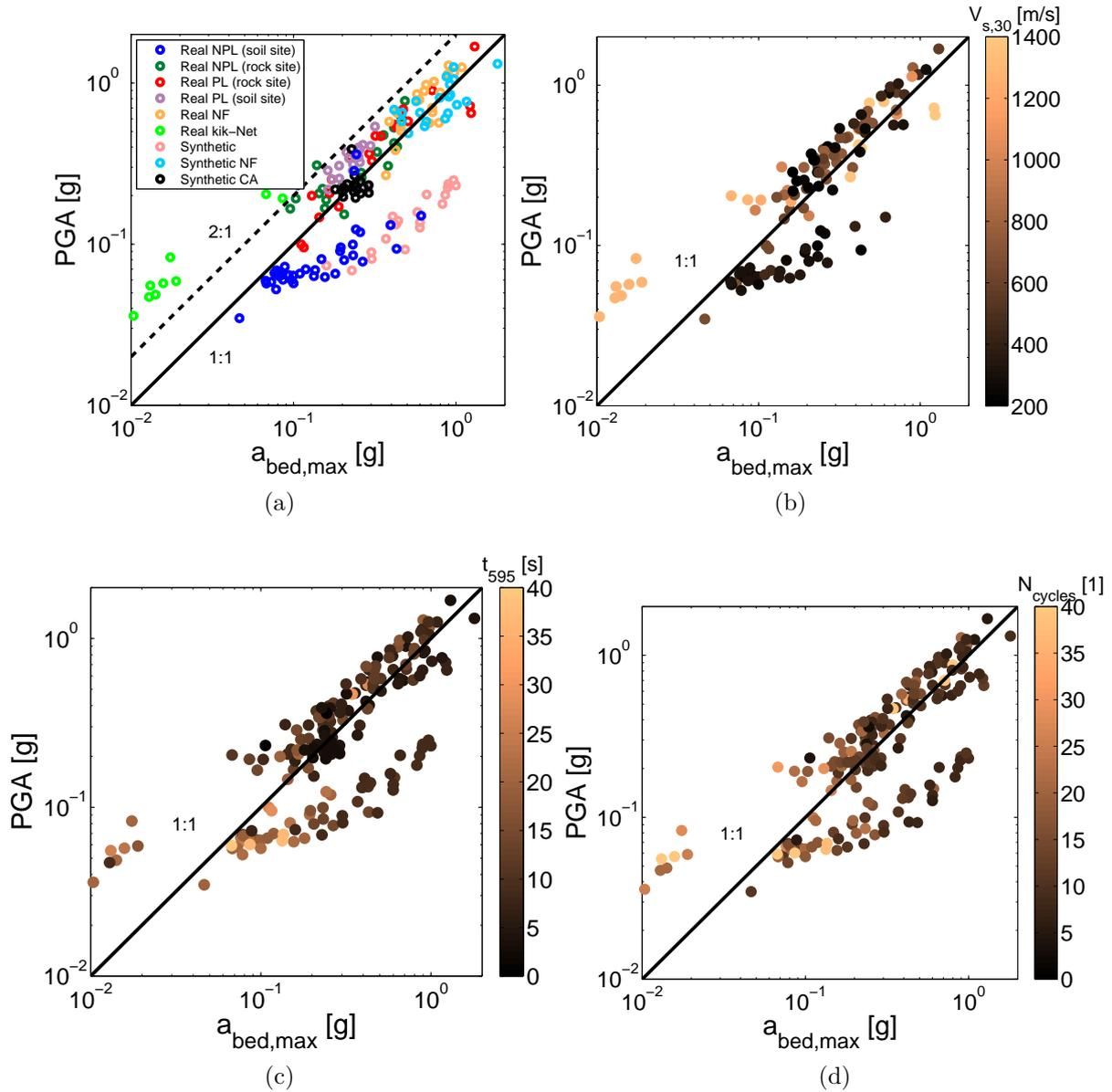
Figure 3.19: PGA at FF classified according to: a) input signal's type, b) shear velocity  $V_{s,30}$  of real motions, c) duration of mainshock  $t_{595}$ , d) number of cycles  $N_{cycles}$  of input signal
