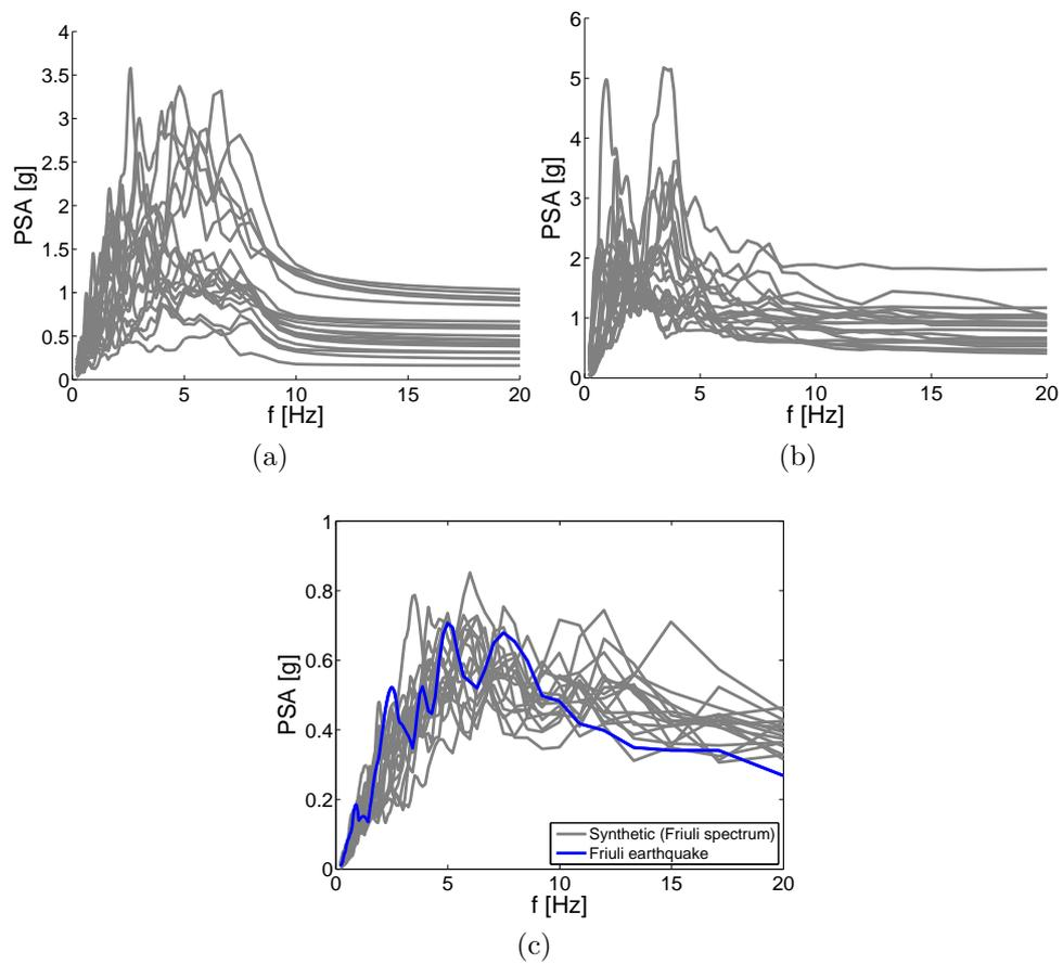
Figure C.16: Acceleration spectrum of synthetic input seismic motions ( $\xi=5\%$ ): a) Strong seismic motions (GV), b) Synthetic near-fault (nfs), c) Generated from Code\_Aster based on the characteristics of Friuli earthquake.
