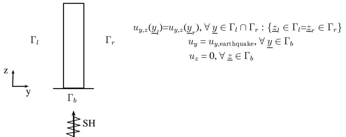
Figure 4.1: S wave propagation in a 9m high dry nonlinear soil column.
