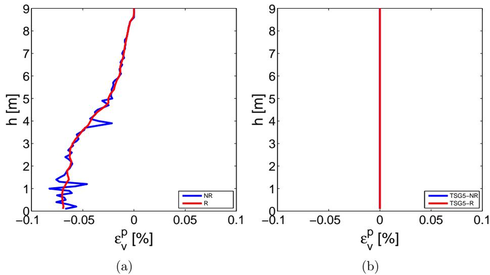
Figure G.18: Profile of plastic volumetric deformations at the end of the input ground motion: a) Zero shear-induced volumetric deformations, b) Isotropic mechanism deactivated and zero shear-induced volumetric deformations.
