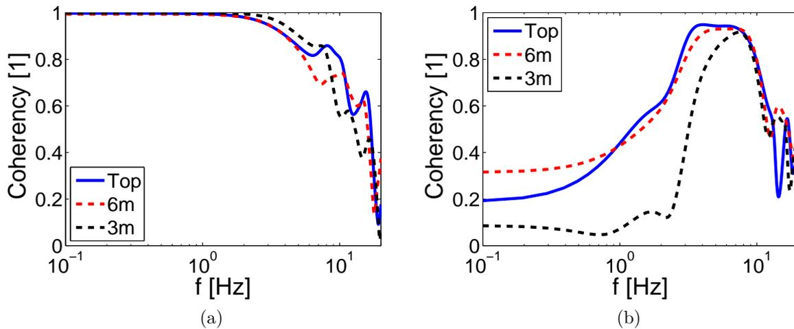
Figure 4.10: Coherency of FF acceleration without and with regularization: a) Horizontal, b) Vertical induced.
