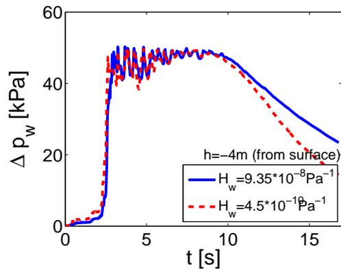
Figure D.12: Influence of water compressibility on soil liquefaction.
