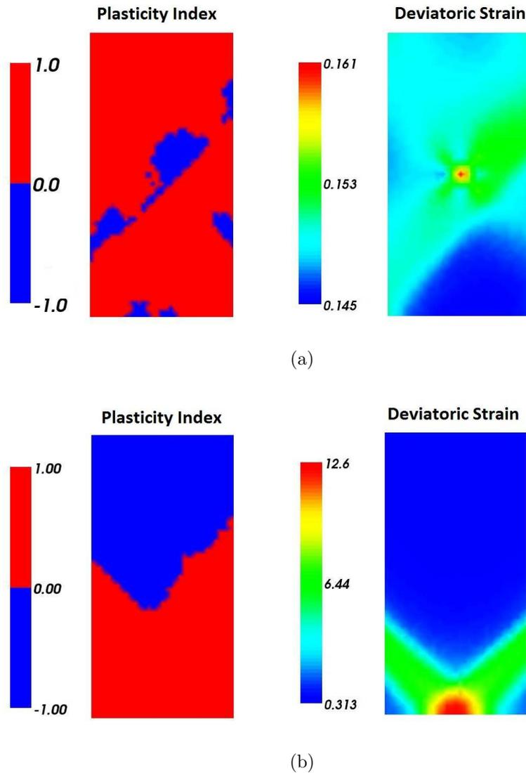
Figure F.6: Biaxial test of Hostun sand (DR=88%) -  $p_0=-500\text{kPa}$ ,  $a_1=1500\text{Pa}\cdot\text{m}^2$ : a)  $t=0.15\text{s}$  ( $u_v=0.024\text{m}$ ), b)  $t=2\text{s}$  ( $t_{end}$ ,  $u_v=0.32\text{cm}$ ).
