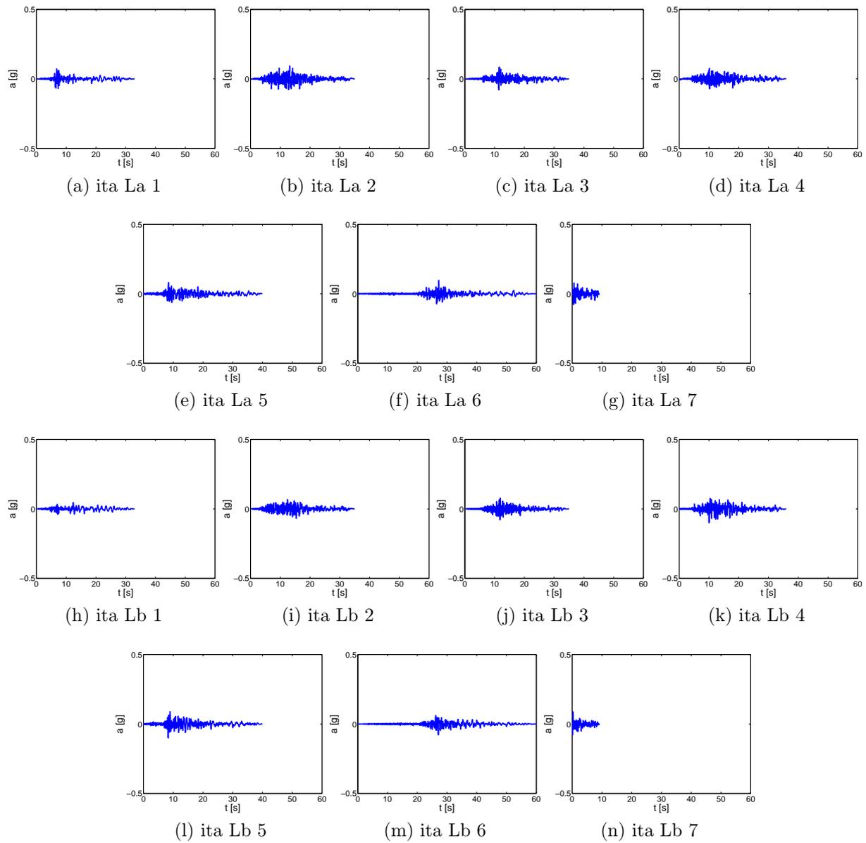
Figure C.2: Accelerograms of low non pulse-like real earthquakes recorded on soil site.
