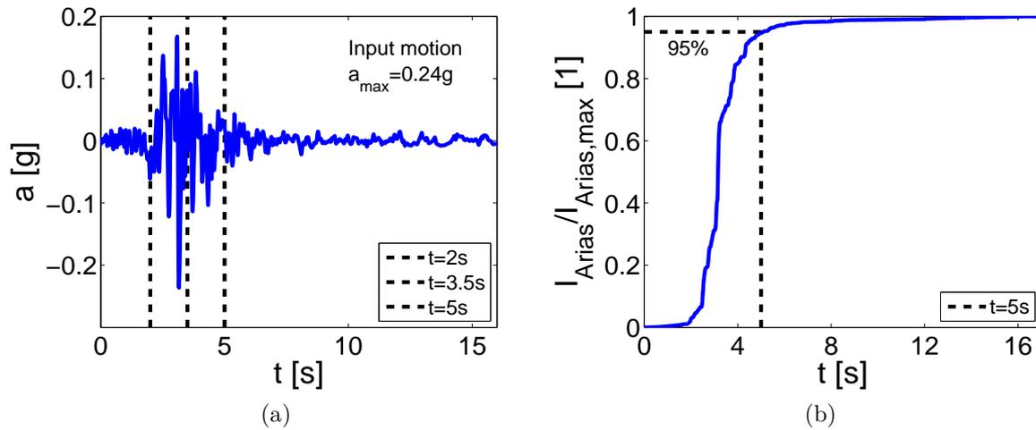
Figure 5.5: Input seismic signal of Friuli earthquake: a) Accelerogram, b) Normalized Arias intensity.
