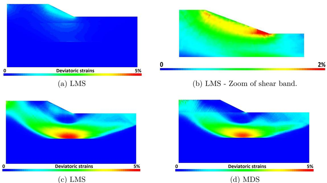
Figure 5.32: Deviatoric strains  $\varepsilon_d$  at the end of Friuli earthquake: a,b) Fully drained effective stress simulation, c,d) Coupled effective stress simulation.
