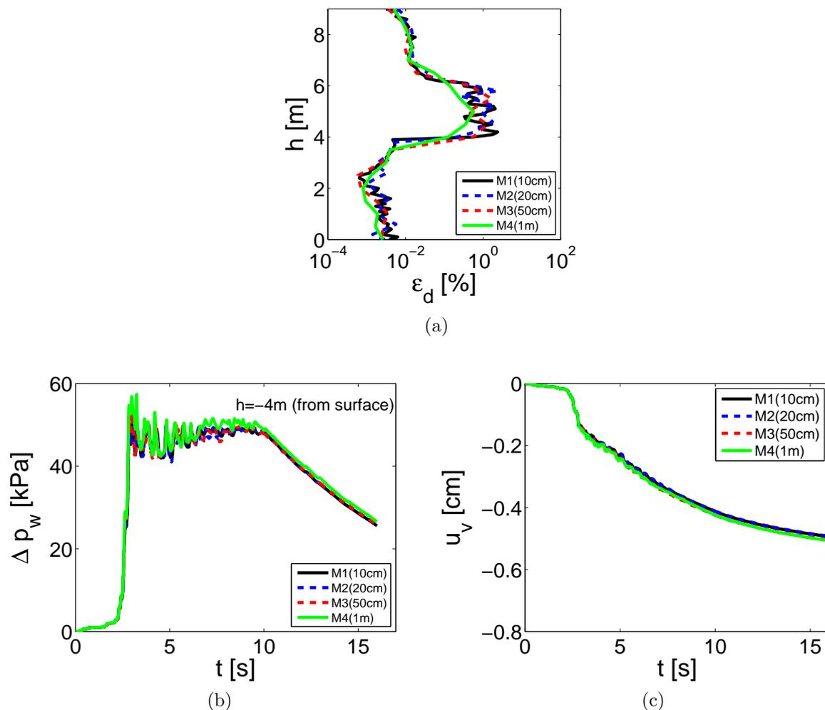
Figure 3.15: Mesh dependency evaluation of dynamic response with different meshes as obtained by Code\_Aster : a) Profile of deviatoric strains ( $\varepsilon_d$ ) at the end of the ground motion, b) Excess pore water pressure evolution, c) Ground surface settlement evolution.
