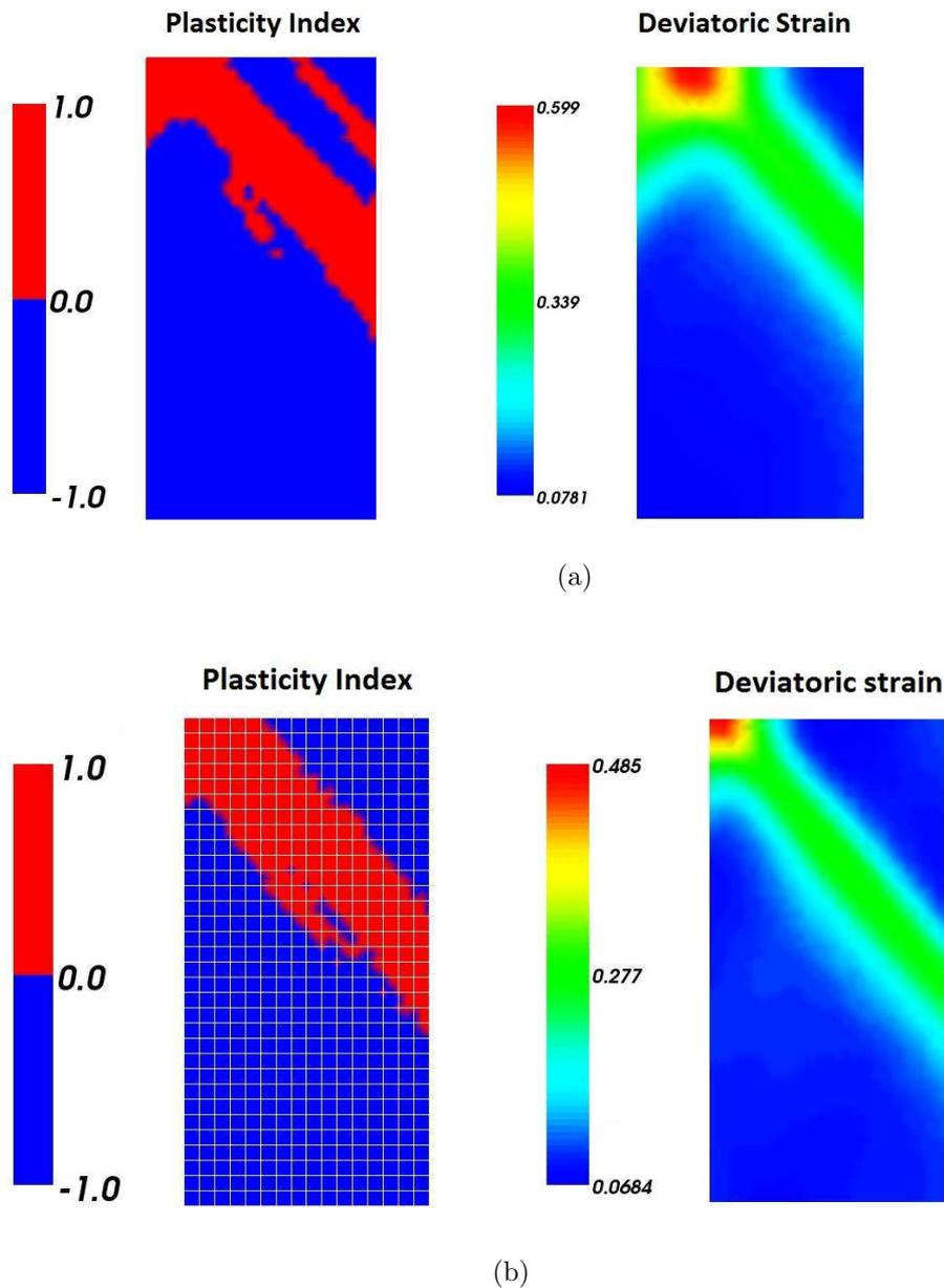
Figure F.9: Biaxial test of Hostun sand (DR=88%) with  $p_0 = -100 \text{ kPa}$ : a)  $a_1/25 = 26 \text{ Pa} \cdot \text{m}^2$ ,  $t = 0.63 \text{ s}$  ( $t_{end}$ ,  $u_v = 0.025 \text{ m}$ ), b)  $a_1/50 = 13 \text{ Pa} \cdot \text{m}^2$ ,  $t = 0.48 \text{ s}$  ( $t_{end}$ ,  $u_v = 0.02 \text{ m}$ ).
