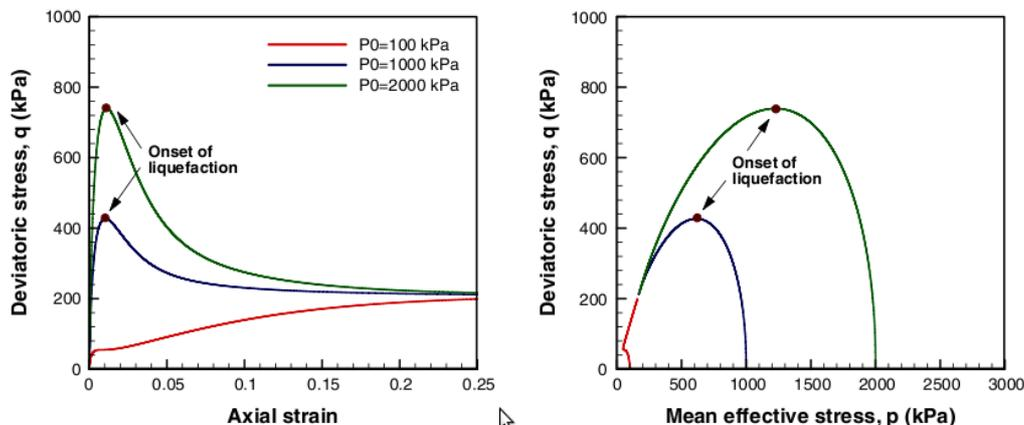
Figure 2.7: Numerical results of undrained triaxial compression test on samples of loose Toyoura sand (Mohammadnejad and Andrade, 2014).
