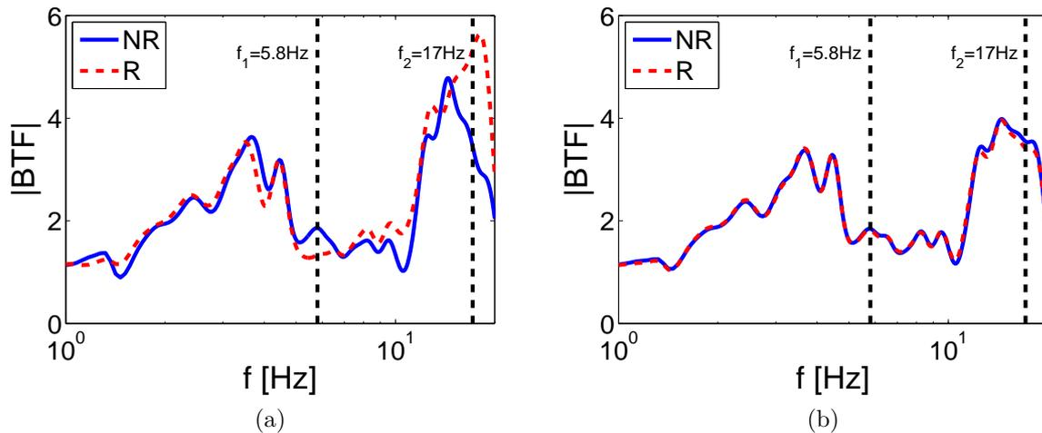
Figure 4.8: Borehole Transfer Function of FF horizontal acceleration: a) Dilatancy rule activated, b) Dilatancy rule deactivated: No shear-induced volumetric strains.
