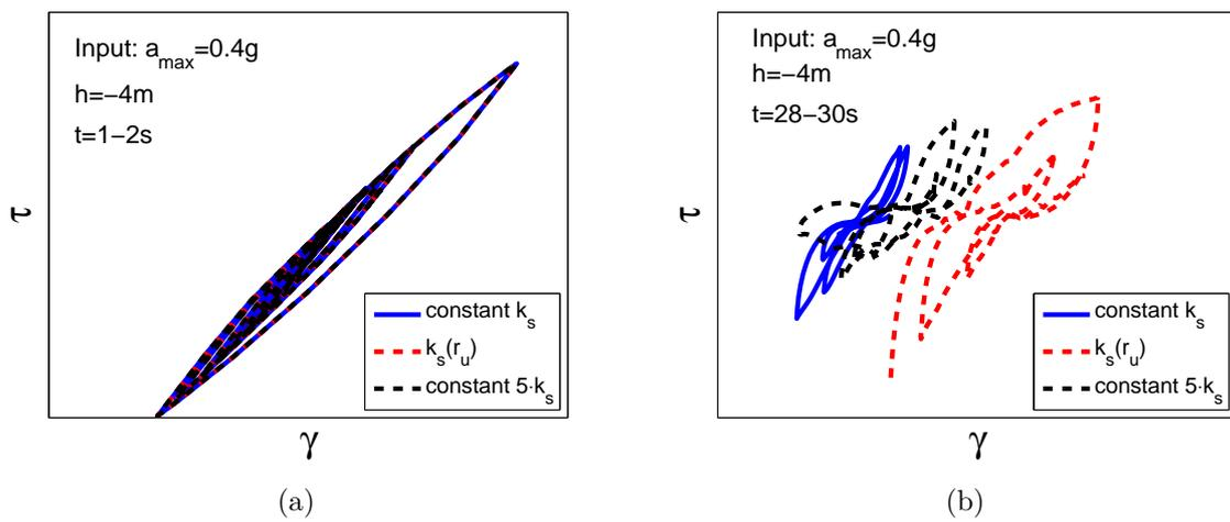
Figure 3.38: Comparison of shear stresses ( $\tau$ ) - shear strains ( $\gamma$ ) of three simulations at  $h = -4\text{m}$  from the surface for the strong input motion ( $a_{\max} = 0.4g$ ): a)  $t = 1-2\text{s}$ , b)  $t = 28-30\text{s}$ .
