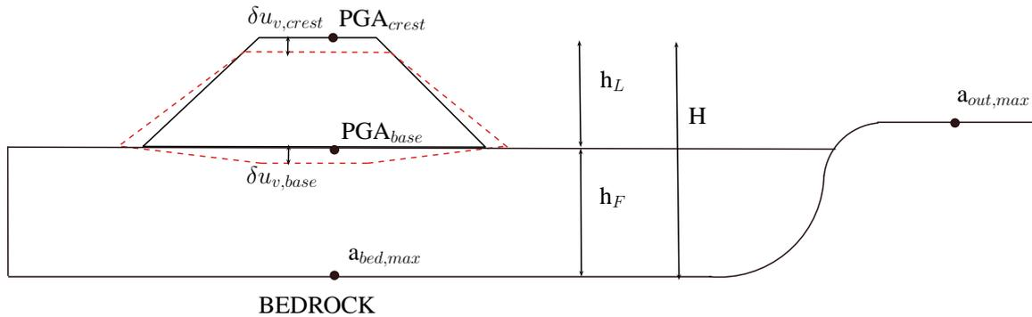
Figure 6.33: Schematic representation of calculation of levee's settlements.
