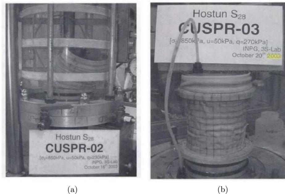
Figure 2.4: Undrained triaxial compression tests on very loose specimens of Hostun sand: a) Total liquefaction, b) Partial liquefaction (Servant et al., 2005).
