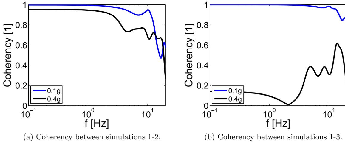
Figure 3.44: Coherency of measured acceleration for all simulations.
