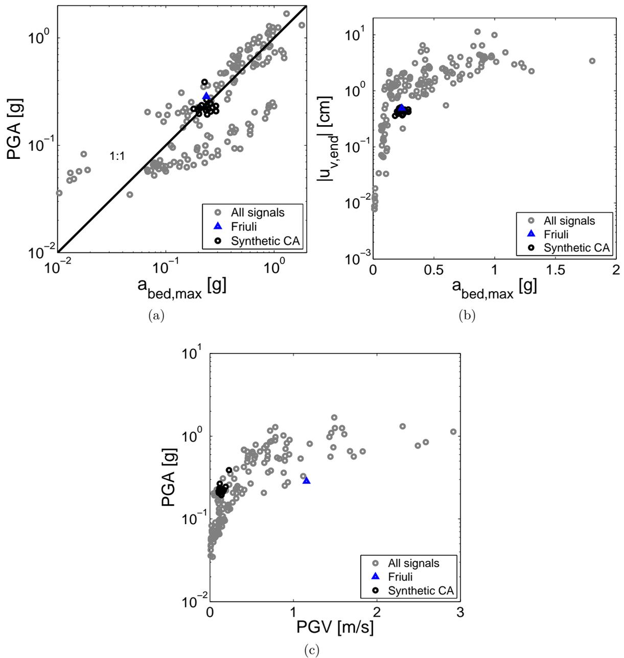
Figure 3.23: Comparison of synthetic motions and Friuli (in grey all other motions): Soil column's response in terms of: a) PGA as function of the input motion  $a_{bed,max}$ , b) Settlements at FF as function of the input motion  $a_{bed,max}$ , c) PGA-PGV at FF.
