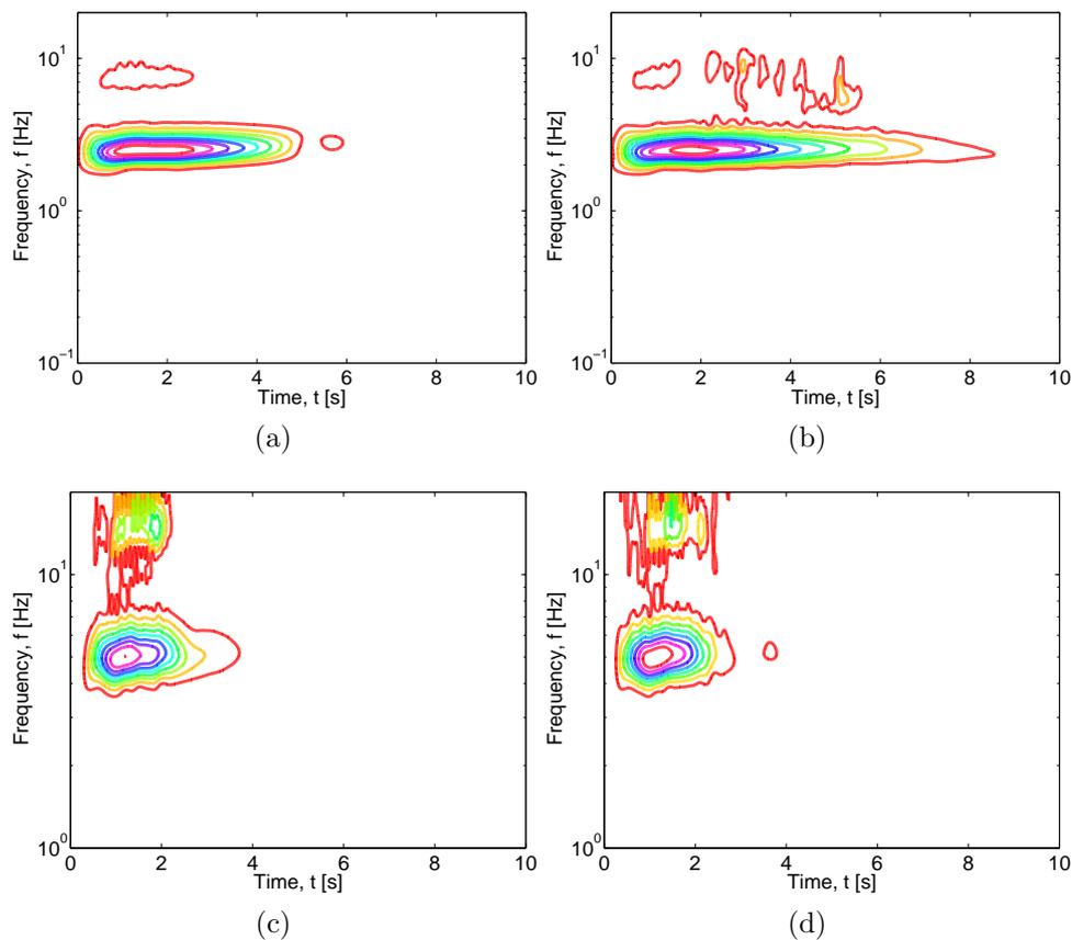
Figure G.4: Comparison of S-transform without and with regularization: a) FF horizontal acceleration-Without regularization, b) FF horizontal acceleration-With regularization, c) Induced vertical acceleration-Without regularization, d) Induced vertical acceleration-With regularization.
