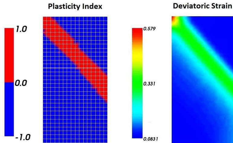
Figure F.7: Biaxial test of Hostun sand (DR=88%):  $p_0=-500\text{kPa}$ ,  $a_1/25=60\text{Pa} \cdot \text{m}^2$ ,  $t=0.15\text{s}$  ( $t_{end}$ ,  $u_v=0.024\text{m}$ ).
