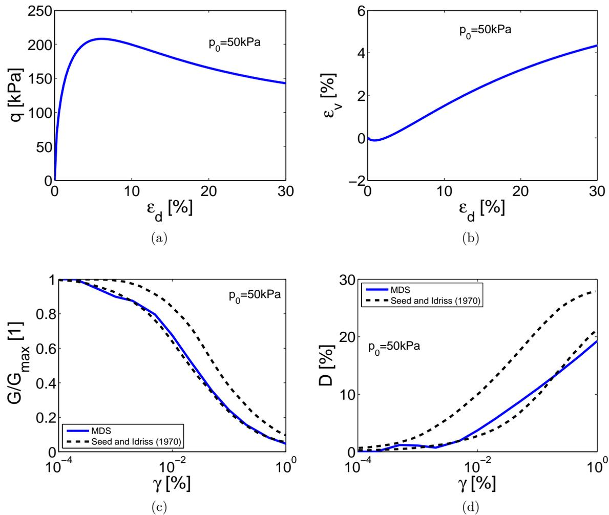
Figure 4.2: Soil response of one material point with the ECP constitutive model ( $p_0=50\text{kPa}$ ,  $K_0=1.0$ ): a,b) Monotonic triaxial drained test, c,d) Cyclic shear test compared to Seed and Idriss (1970) results.
