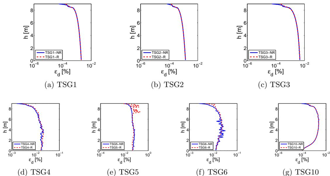
Figure G.2: Profile of deviatoric strains  $\varepsilon_d$  at the end of the input motion.
