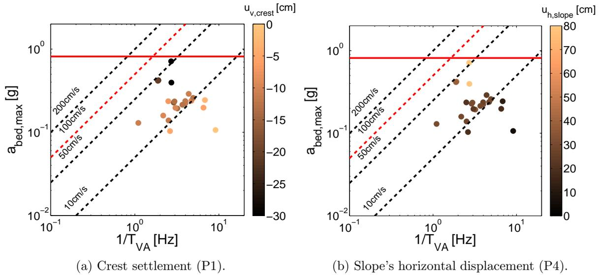
Figure 6.32: Relative to FF displacements classified according to the relation between input IM:  $a_{bed,max}$  and  $T_{V,A}$ .
