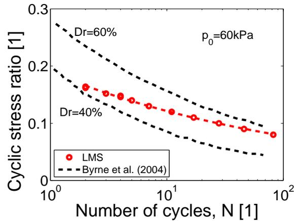
Figure 5.22: Soil response of one material point under triaxial cyclic undrained test: Liquefaction curve compared to Byrne et al. (2004).
