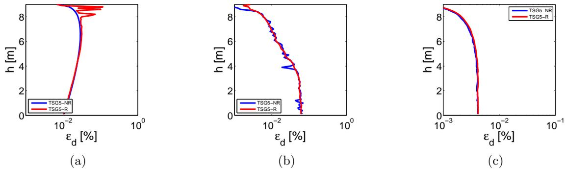
Figure G.13: Profile of deviatoric strains  $\varepsilon_d$ : a) Isotropic mechanism deactivated, b) Zero shear-induced volumetric deformations, c) Isotropic mechanism deactivated and zero shear-induced volumetric deformations.
