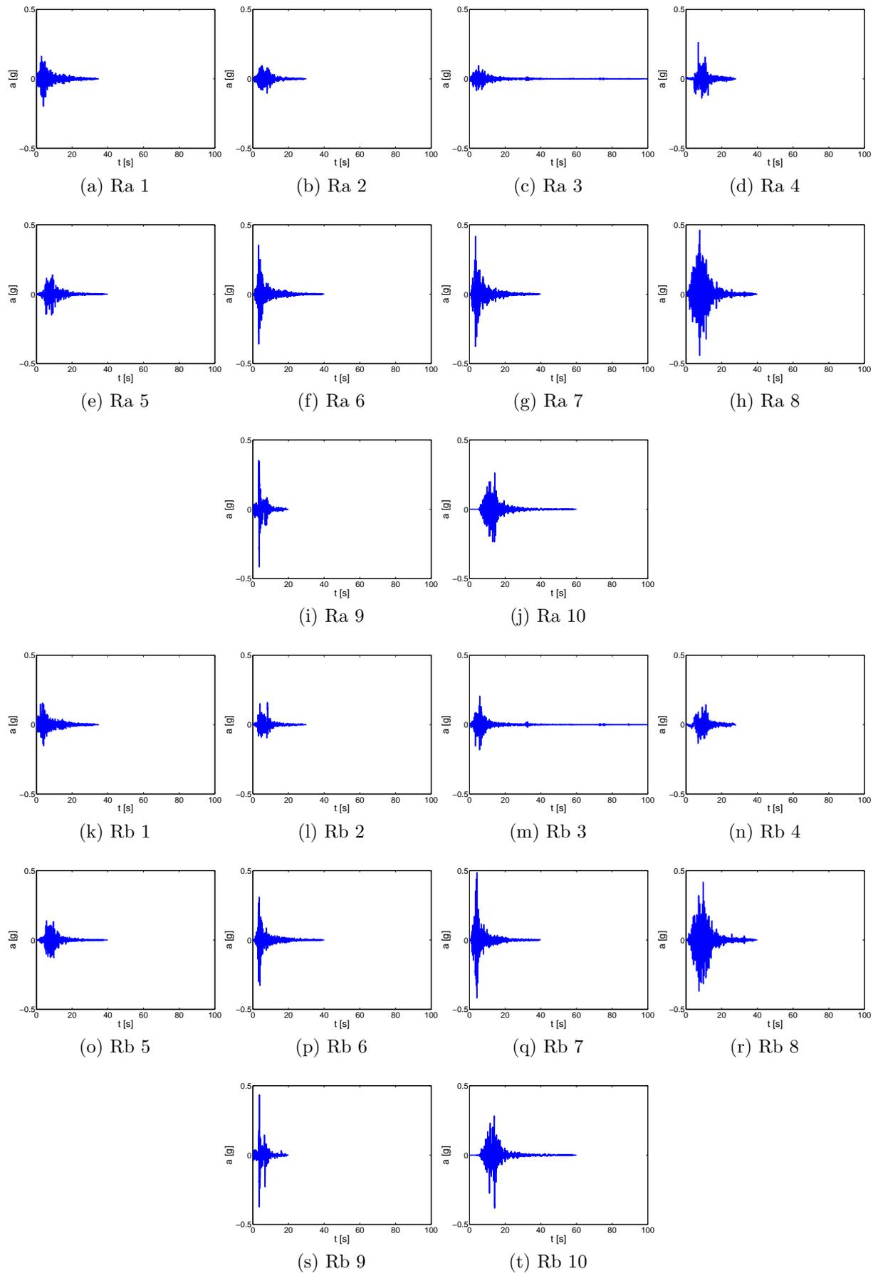
Figure C.4: Accelerograms of non pulse-like real earthquakes recorded on rock site.
