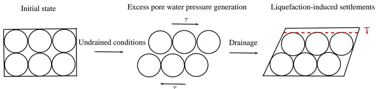
Figure 2.3: Soil liquefaction.
