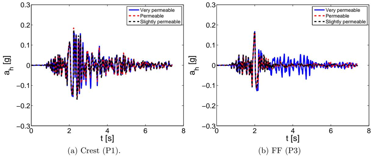
Figure 6.23: Influence of soil's permeability (irsn168): Horizontal acceleration.
