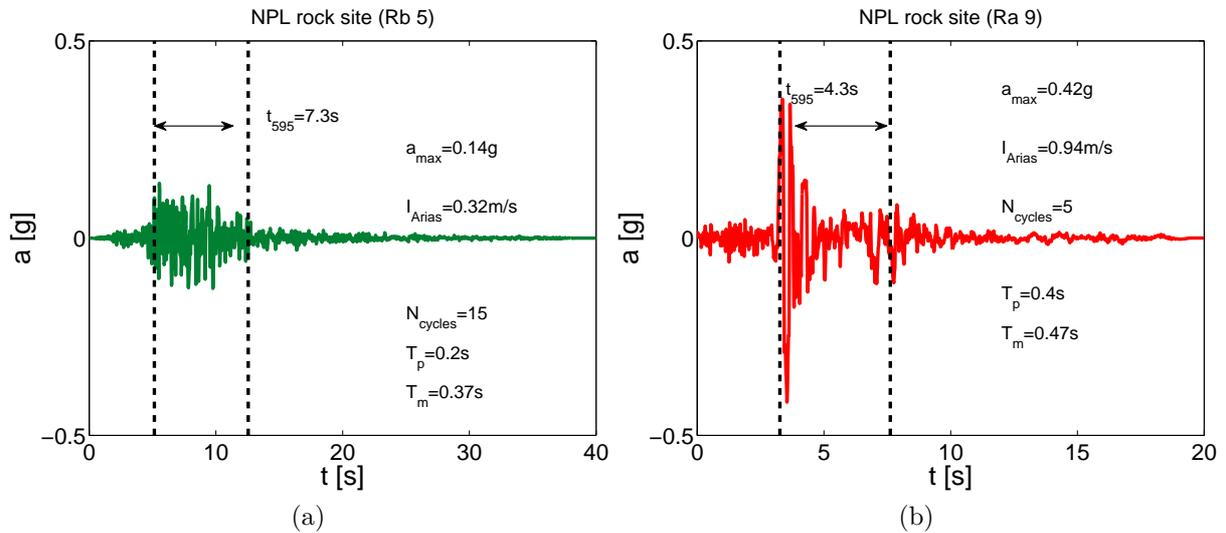
Figure 6.30: Input ground motions: a) Low (Rb 5), b) Strong (Ra 9).
