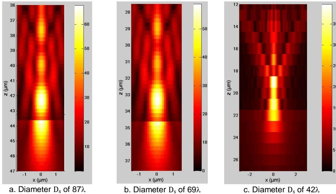
Figure 3.21. The total electric field distribution in XZ plane for a barium-titanate microspheres ( $n_{\text{BaTiO}_3} = 1.9$ ) with a diameter  $D_s$  of (a)  $87\lambda$ , (b)  $69\lambda$  and (c)  $42\lambda$
