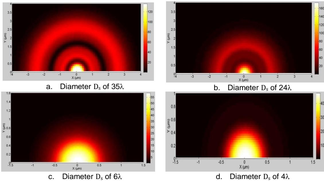
Figure 3.39. Intensity ( $I = |E|^2$ ) in the plane parallel to the OXY plane and tangent to the sphere for glass microspheres having diameter  $D_s$  of (a)  $35\lambda$ , (b)  $24\lambda$ , (c)  $6\lambda$  and (d)  $4\lambda$
