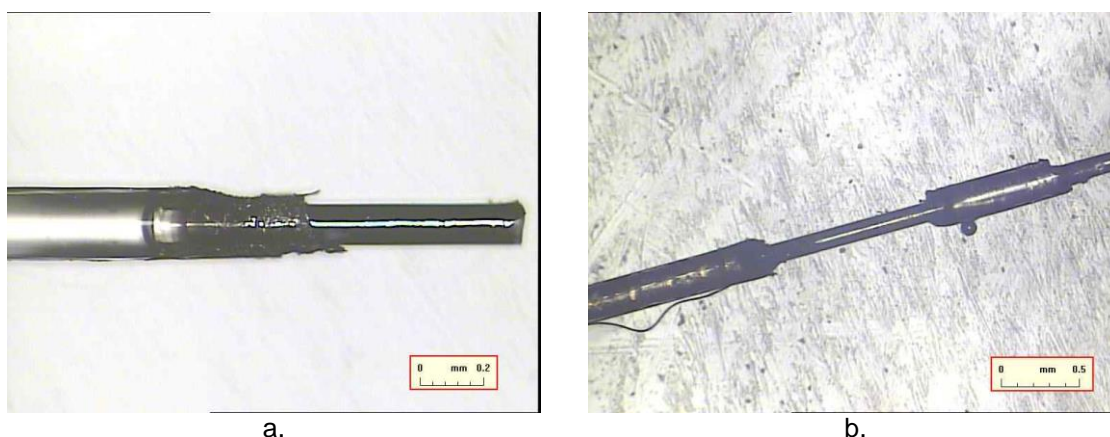
Figure 4.62. Thermal effects of laser injection burnt/melt SMF28 cladding, (a) at the jacket beginning and (b) near the jacket beginning
