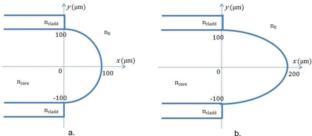
Figure 4.55. Geometrical design of MMF 200 μm core optical fiber in 2D:
