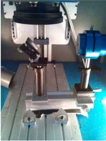
Figure 3.25. Setup to measure the beam profile of the YLIA M20 Quantel fiber laser system; the laser comes out from the galvanometer head is filtered and reflected into the NanoScan™ sensor.
