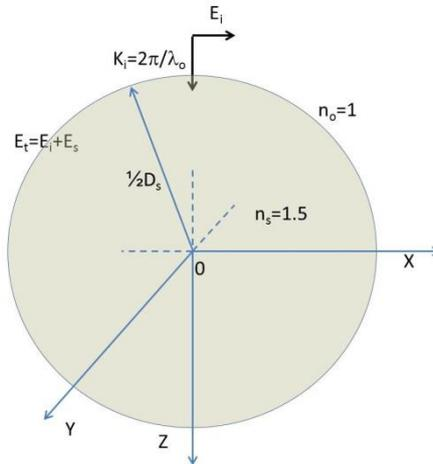
Figure A.71. Spherical polar coordinate center inside a sphere of diameter  $D_s$
