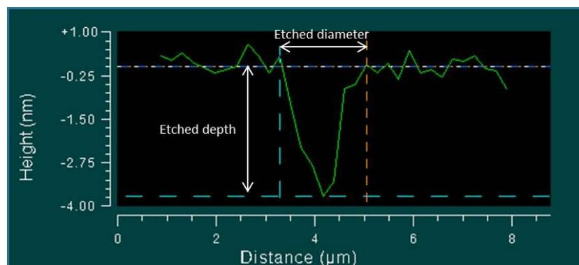
Figure 3.33. An etching mark profile with its parameters
