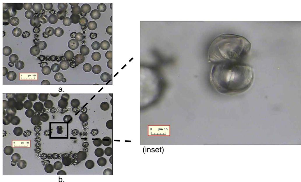
Figure 3.41. Barium-titanate microspheres ( $D_s = 69 \mu\text{m}$ ) on silicon wafer (a) before and (b) after laser illuminations with (inset) a broken microsphere inside the cell ( $F_z = 0.7 \text{ J/cm}^2$ ).
