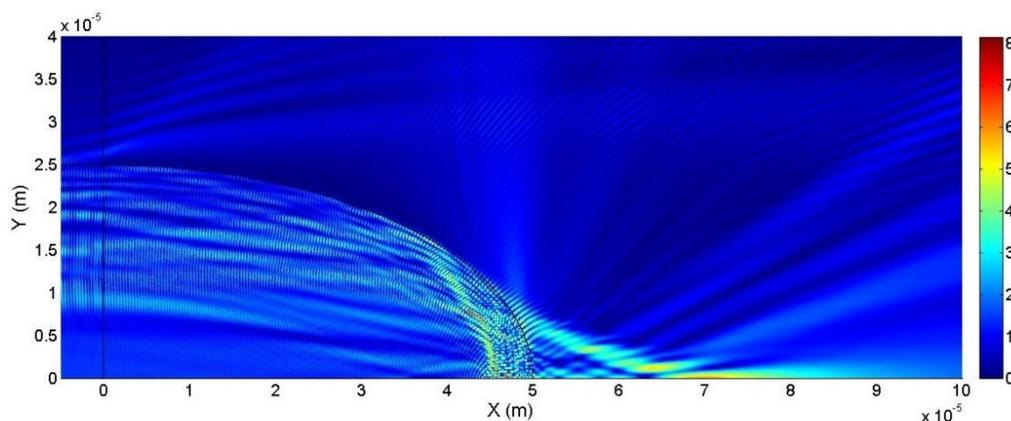
Figure 4.53. Total electric field of a half planar waveguide ( $D_s = 50 \mu\text{m}$ ) with an elliptical tip ( $b = 2a$ ,  $\text{NA} = 0.17$ )
