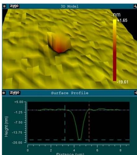
Figure 3.34. The smallest PJ etching on silicon wafer using a glass microsphere  $D_s = 6 \mu\text{m}$  ( $F_z = 0.7 \text{ J/cm}^2$ )
