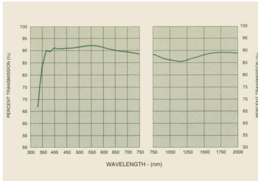
Figure A.72. Soda lime glass transmission as a function of wavelength is taken from S. M. Company. (2013, 14 June 2013). Optical transmission curve is available at <http://www.sinclairmfg.com/datasheets/optical3.html>
