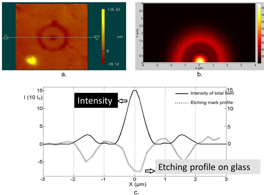
Figure 3.40 The correlation between total intensity distribution map and PJ etching profile on glass in the case of glass microspheres  $D_s$  of  $24\mu\text{m}$ ; (a) A PJ etching taken by Zygo®. (b) The intensity distribution map on the surface. (c) The correspondence between PJ etching profile and intensity profile.
