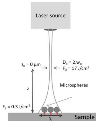
Figure 3.22. The laser illumination scheme
