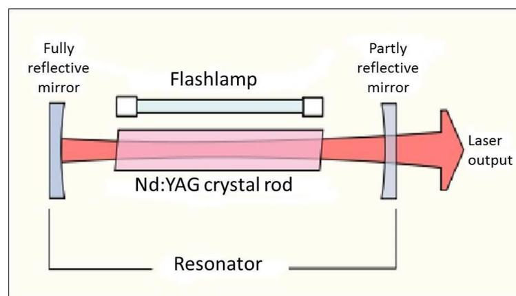
Figure 1.3. The simplified construction of Nd:YAG laser
