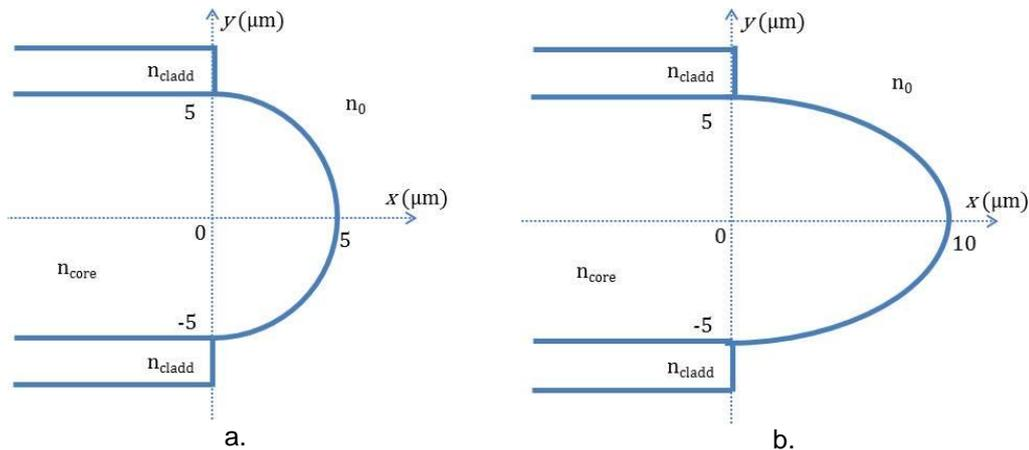
Figure 4.47. Geometrical design of SMF-28,  $10\ \mu\text{m}$  optical fiber core diameter in 2D: (a) circular tip and (b) elliptical tip ( $b = 2a$ )
