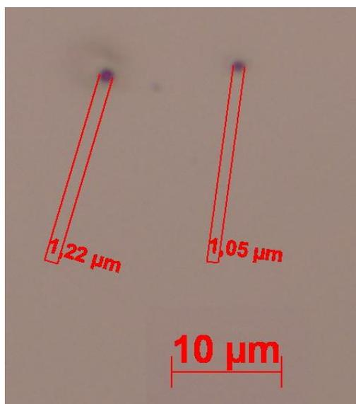
Figure 4.70. Smallest etching obtained with the 100  $\mu\text{m}$  core silica optical fiber with a spheroid tip (NA = 0.22) at  $f = 100 \mu\text{m}$  and with 35 pulses.
