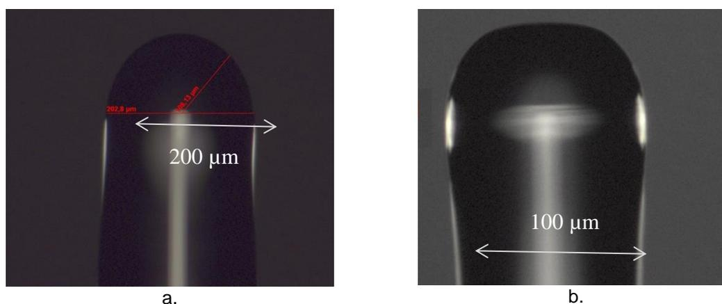
Figure 4.59. The spheroid tipped of (a) our TEQS<sup>TM</sup> coated multi-mode 200  $\mu\text{m}$  fiber and (b) 100  $\mu\text{m}$  silica fiber fabricated by Lovalite for our experiments
