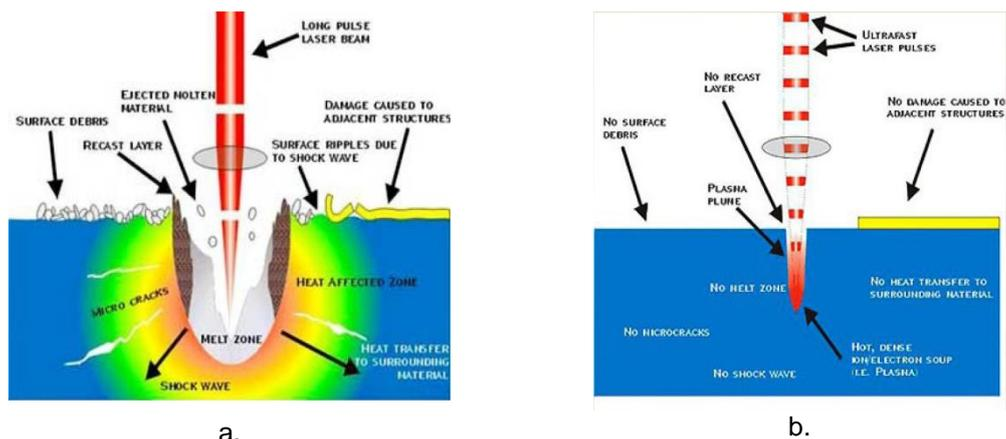
Figure 1.2. Schematic illustration of the ablation process under (a) long pulse and (b) ultrafast laser beam (the figures are taken from [www.aoficorp.com](http://www.aoficorp.com))
