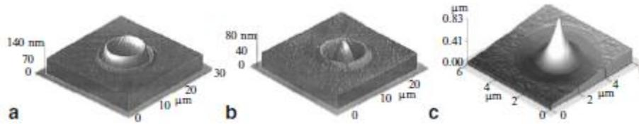
Figure 1.1. AFM images of the surface deformation recorded on Ni-P hard-disk substrate at (a) high energy, (b) intermediate energy [31] and (c) 0.8  $\mu\text{m}$  nano-tip formed on Si – silicon on insulator [32]
