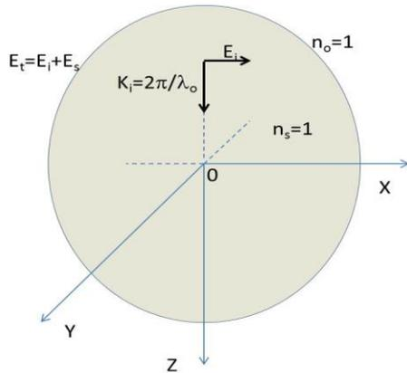
Figure 3.19. A sphere in free space is illuminated by a plane wave ( $E_x, H_y, k_z$ ). The incident wave propagates in the  $+z$  direction
