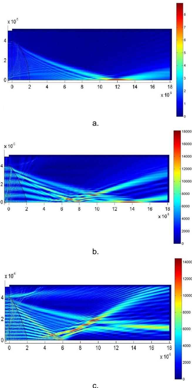
Figure 4.67. Total electric field of a half planar waveguide ( $D_s = 80 \mu\text{m}$ ) with a sharp-curvature end (Bezier weight = 0.405, tip-length =  $20 \mu\text{m}$ ) for different excited mode: (a) fundamental mode, (b) mode 5 and (c) mode 13.
