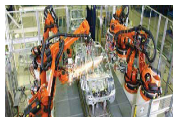
(c) Cooperative manipulators for spot welding by KUKA® systems [279].
