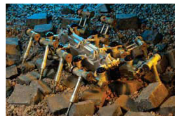
(d) Eight-legged walking robot (Scorpion) for space exploration developed by University of Bremen - Germany.
