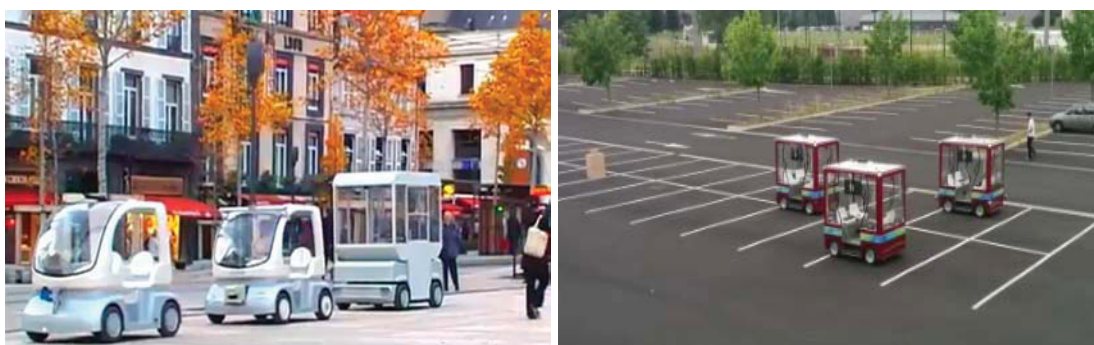
Figure 5.1: Autonomous navigation in formation of a group of UGVs in an urban environment (Clermont-Ferrand, France).
