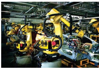
(a) Industrial robot (FANUC®) for car manufacturing [263].
