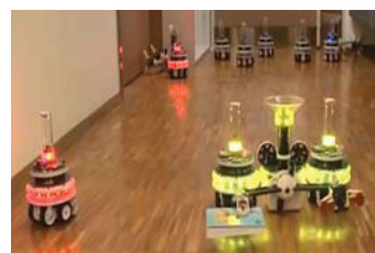
(f) Heterogeneous small autonomous robots dynamically connected by Swarmanoid project [322].
