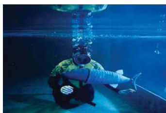
(c) Fish robot (MIT®) named RoboTuna.
