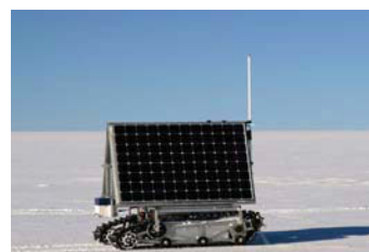
(d) Polar rover robot (NASA®) named Goddard Remote Operated VEHICLE (GROVER).
