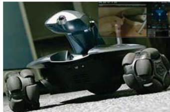
(a) Rovio for Wi-fi enabled surveillance developed by WowWee®.
