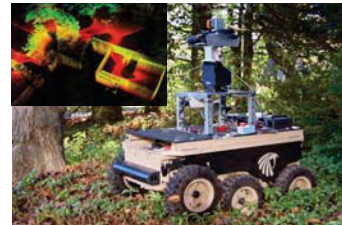
(b) Landshark UGV (Black-i Robotics) with complex mapping sensor system developed by SRI®.
