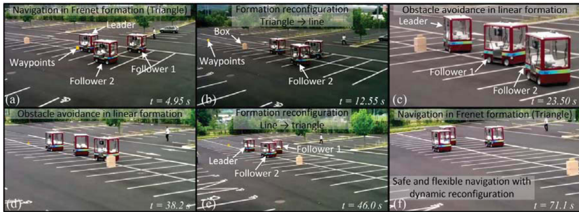
Figure 5.24: Navigation with reconfiguration (SFR-D) in Frenet formation for a group of N = 3 UGVs.
