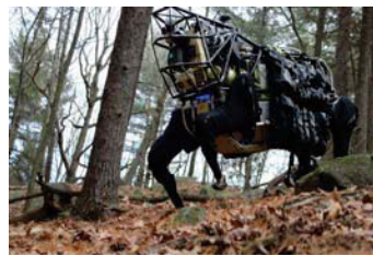
(b) Quadruped robot (Boston Dynamics®) for soldier assistance in rough terrains [360].
