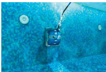
(d) Suction robots (Maytronics®) for cleaning of swimming pool [381].
