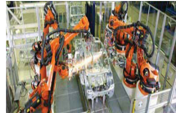
(c) Cooperative manipulators for spot welding by KUKA® systems [279].
