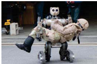
(c) Battlefield Extraction-Assist Robot (BEAR) for search and rescue developed by Vecna Technologies®.
