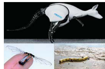
(f) Kangaroo robot (Festo®), Insect fly robot (Harvard) and Salamander robot (EPFL) [257].
