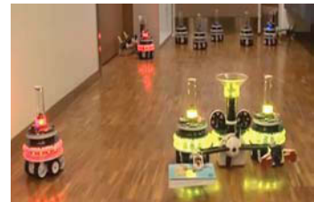
(f) Heterogeneous small autonomous robots dynamically connected by Swarmanoid project [322].
