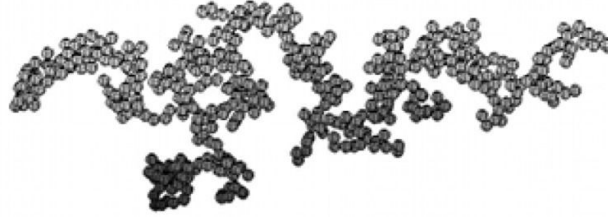
Figure 2.8: Example of hydrocarbon emitted soot, generated using DLCCA, D_f = 1.7 , k_f = 2.0 , N_p = 500
