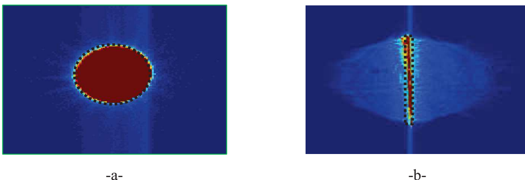
Figure 5.11: Optical measurements of the light power intensity using the beam analyzer. a- Light power intensity over the area of laser beam. b- Light power intensity at the focal point and at the first diffraction order.
