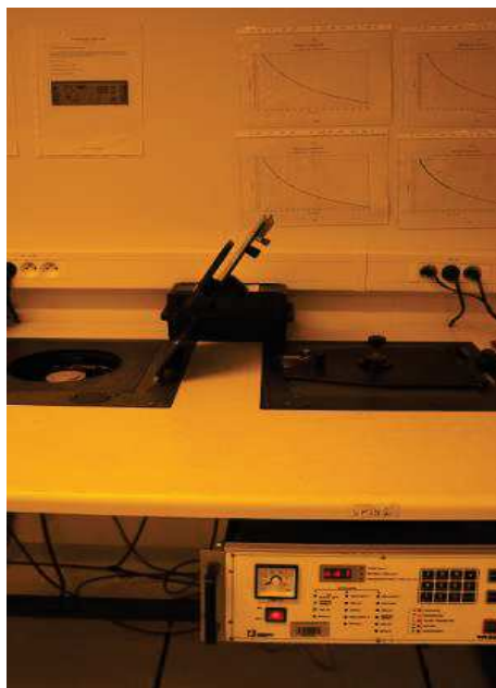
Figure 5.4: The basic setup of the parallel direct writing lithography bench.
