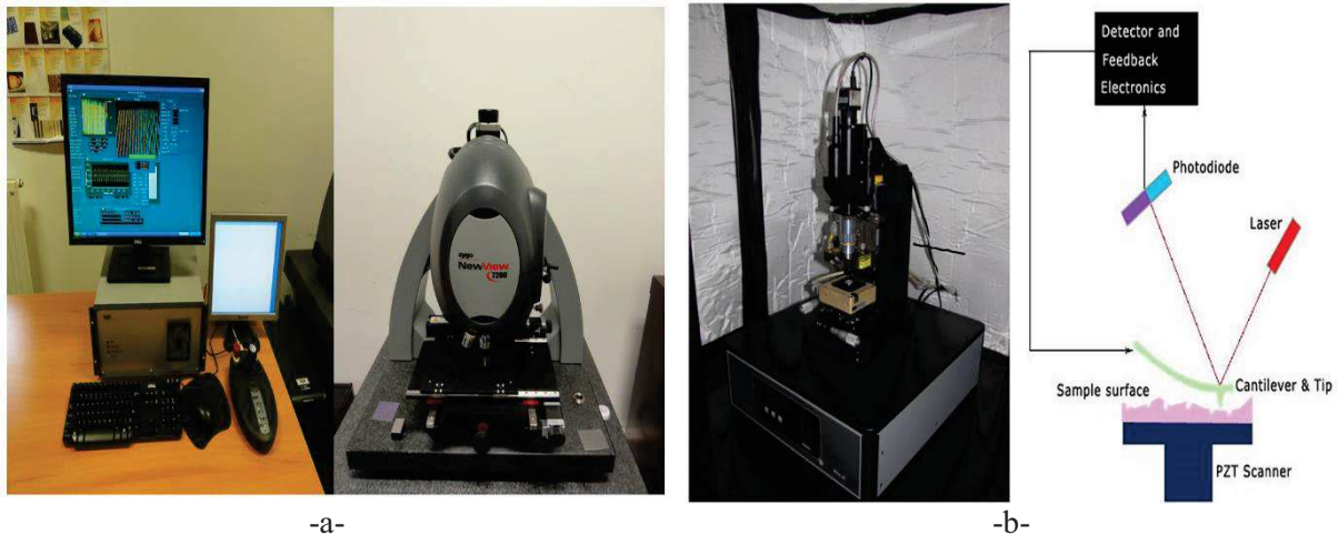
Figure 5.7: Instruments used for the profilometer measurements of the fabricated DOE's: a- Zygo NewView 7200 Optical Profiler. b- Atomic Force Microscope and its working principle.
