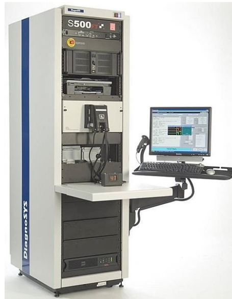
Figure 4.2: Automated RF test equipment ATE500 developed by DiagnoSYS
