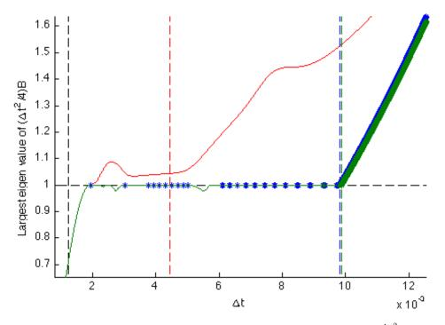
Figure 3.6: Evolution with or without halo of the largest eigenvalue of  $\frac{\Delta t^2}{4}B$  according to  $\Delta t$  for a spatial refinement  $p_s = 8$  (the legend is the same as for Figure 3.3).
