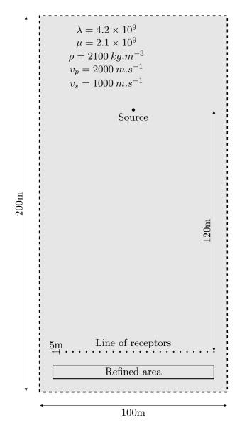
Figure 3.17: Homogeneous medium characteristics.
