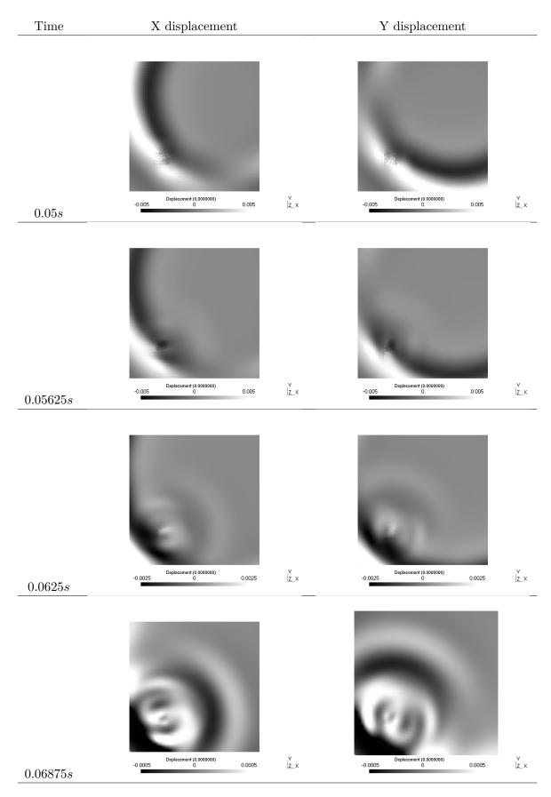
Figure 4.17: Snapshots at different times of X and Y displacement for a medium with diffracting points.
