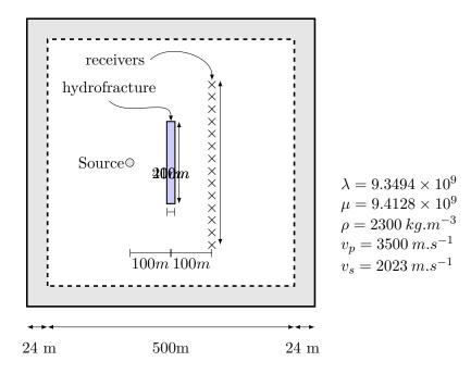
Figure 4.9: Medium with large hydrofracture characteristics.
