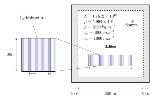
Figure 4.19: Corridor of hydrofractures medium characteristics.
