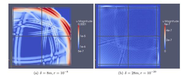
Figure 2.8: Magnitude of the displacement amplified by a factor of 1000 for different PML thickness at T = 0.30s, for an homogeneous medium with  $\rho = 2300 kg.m^{-3}$ ,  $\lambda = 7.774 \times 10^9$  and  $\mu = 3.887 \times 10^9$ .
