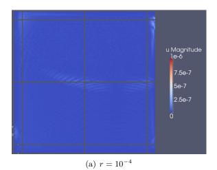
Figure 2.12: Magnitude of the displacement for a color scale divided by a factor of  $1/r = 10^4$  at T = 0.5s, for an heterogeneous medium (see figure 2.10).
