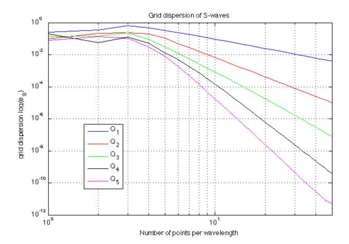
Figure 1.5: Dispersion convergence for S-waves for different polynomial basis according to the number of points per wavelength  $\frac{1}{\varkappa}$ .
