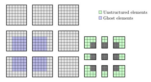
Figure 5.5: Representation of the different subdomains for parallelization.
