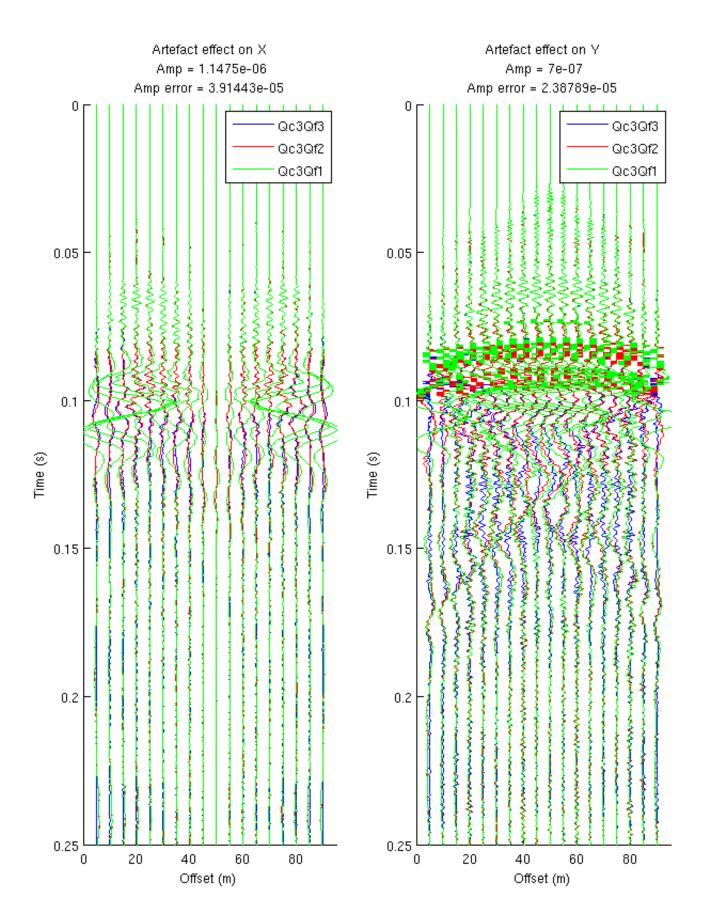
Figure 3.22: Spurious effects  $(u_{ref} - u_h)$  for  $Q_3$  coarse elements and  $Q_3, Q_2, Q_1$  fine elements and with temporal refinement pt = 20 and spatial refinement ps = 20.
