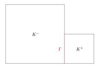
Figure 5.1: Two non-conforming elements.
