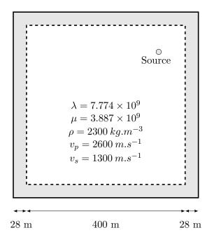
Figure 2.4: Homogeneous medium characteristics.
