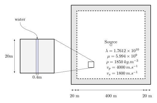
Figure 4.13: Fluid-filled crack medium characteristics.
