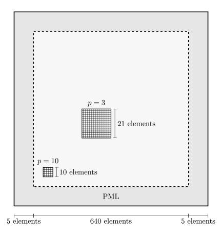
Figure 5.14: Representation of the mesh used for the realistic case performance tests.
