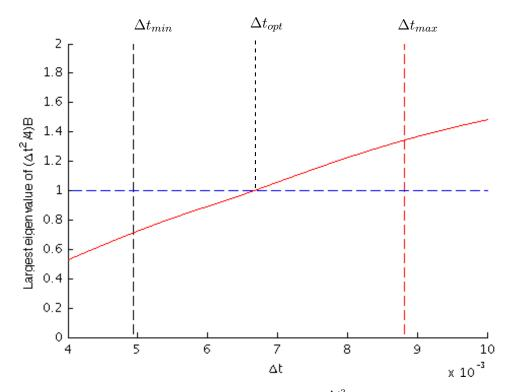
Figure 3.2: Evolution of the largest eigenvalue of  $\frac{\Delta t^2}{4}B$  according to  $\Delta t$  for a spatial refinement  $p_s = 2$ .
