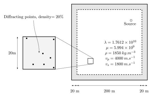
Figure 4.15: Diffracting points medium characteristics.
