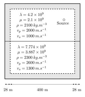
Figure 2.10: Heterogeneous medium characteristics.
