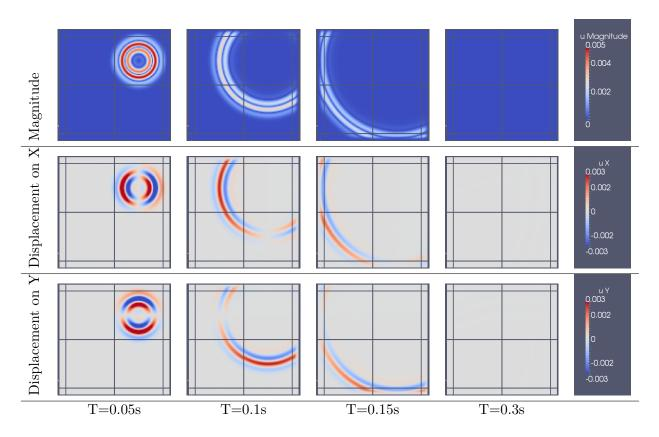
Figure 2.5: Magnitude and amplitude of the displacement at different times, for an homogeneous medium with  $\rho = 2300 kg.m^{-3}$ ,  $\lambda = 7.774 \times 10^9$  and  $\mu = 3.887 \times 10^9$ .
