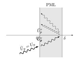
Figure 2.3: Reflection of a plane wave P in a finite PML.
