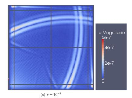
Figure 2.6: Magnitude of the displacement for a color scale divided by a factor of  $1/r = 10^4$  at T = 0.3s, for an homogeneous medium with  $\rho = 2300 kg.m^{-3}$ ,  $\lambda = 7.774 \times 10^9$  and  $\mu = 3.887 \times 10^9$ .
