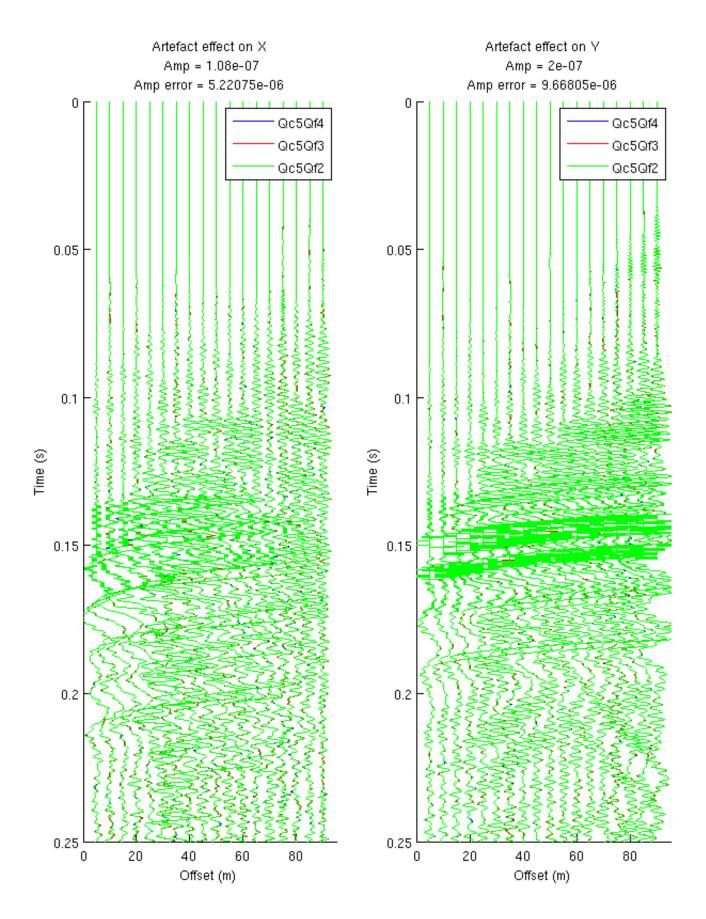
Figure 3.24: Spurious effects  $(u_{ref} - u_h)$  for  $Q_5$  coarse elements and  $Q_4, Q_3, Q_2$  fine elements and with temporal refinement pt = 20 and spatial refinement ps = 20.
