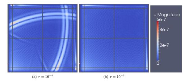
Figure 2.7: Magnitude of the displacement for a color scale divided by a factor of  $10^4$  for different absorption coefficients  $r = 10^{-4}$  and  $r = 10^{-6}$  at T = 0.3s, for an homogeneous medium with  $\rho = 2300 kg.m^{-3}$ ,  $\lambda = 7.774 \times 10^9$  and  $\mu = 3.887 \times 10^9$ .
